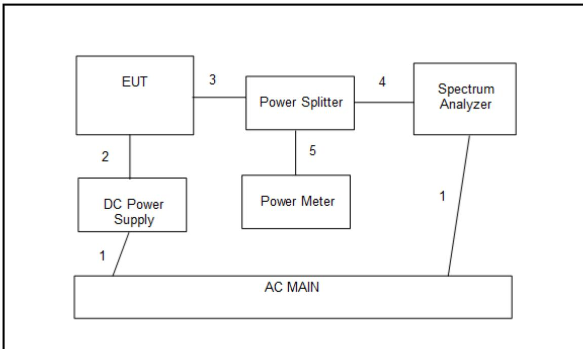
**SETUP DIAGRAM FOR RADIATED TEST**
