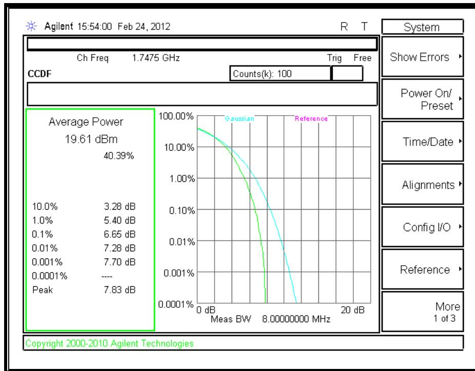
**1732.5MHz, 20MHz QPSK**
