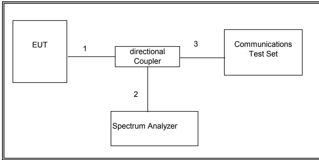
**RADIATED SETUP DIAGRAM FOR TESTS**
