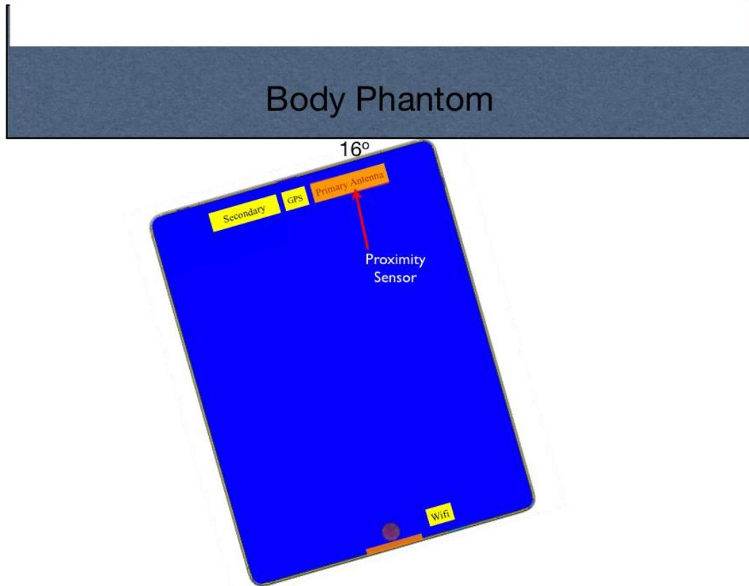
The proximity sensor coverage at the Rear Surface/Right-corner of the device is determined by changing the angle of the device relative to the phantom and observing the angle at which the proximity sensor is no longer triggered. In this case, the conservative angle at which proximity sensor stops triggering is at 20°.
