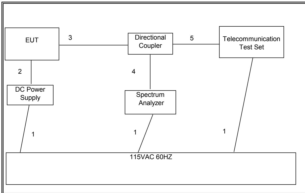
**SETUP DIAGRAM FOR RF RADIATED TESTS**
