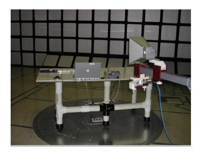
Digital Device Radiated Emission Measurement
