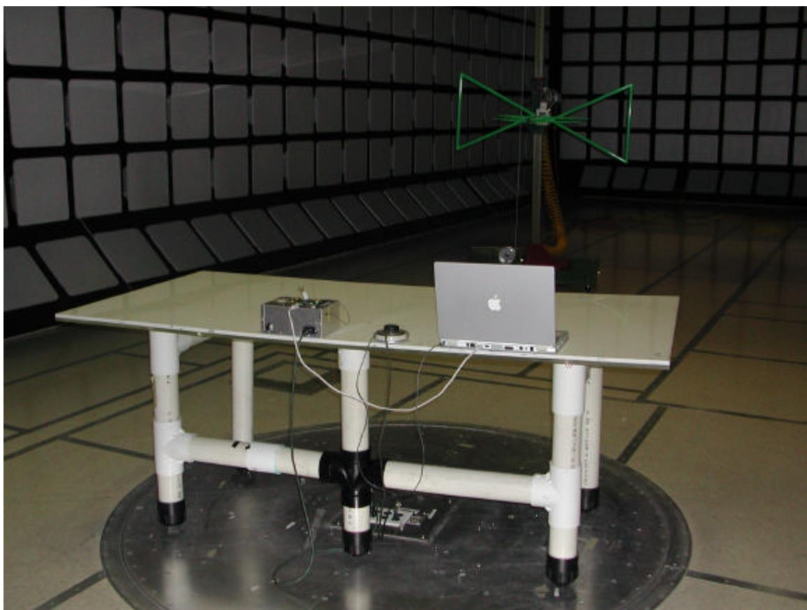
Digital Device Radiated Emission Measurement
