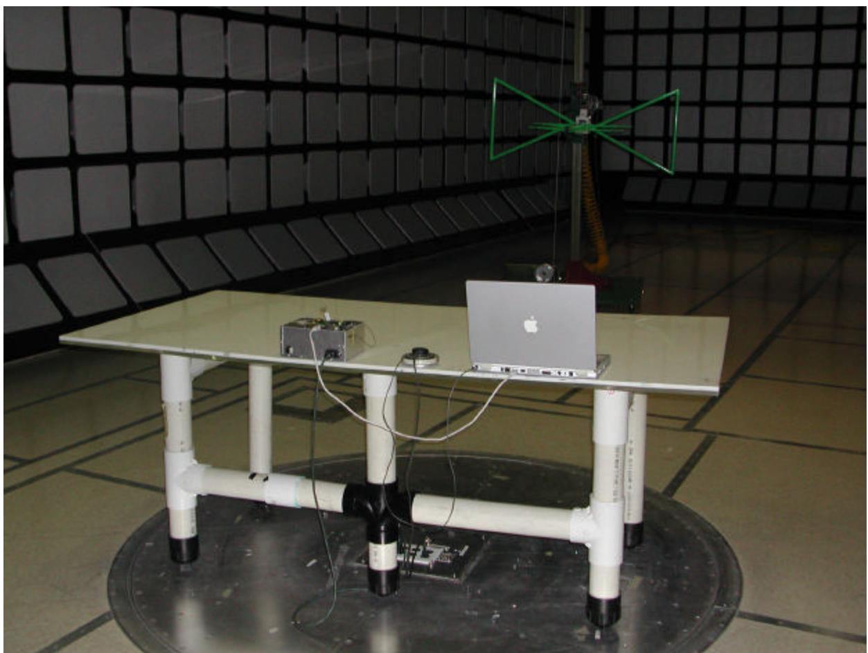
Powerline Conducted Emissions Measurement
