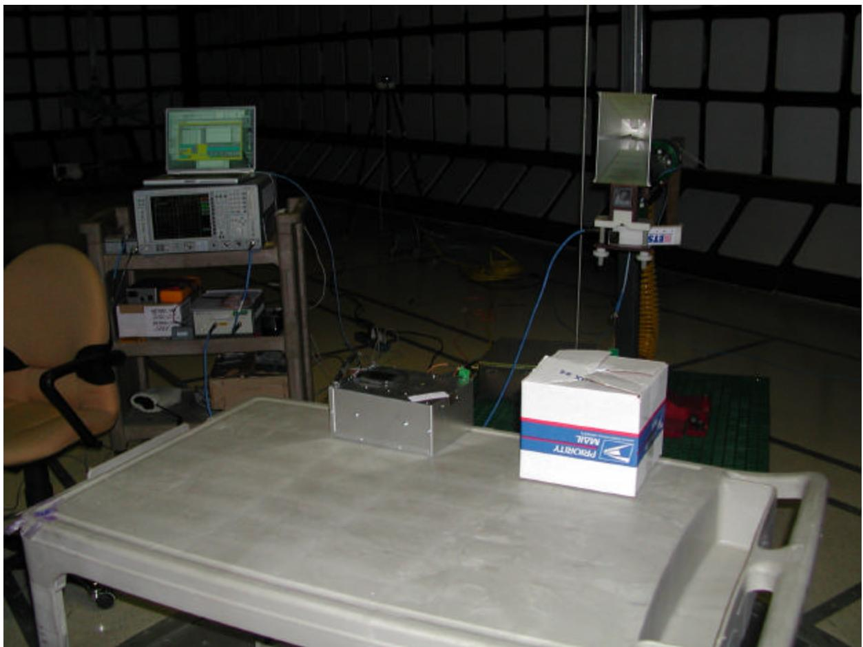
Digital Device Radiated Emission Measurement
