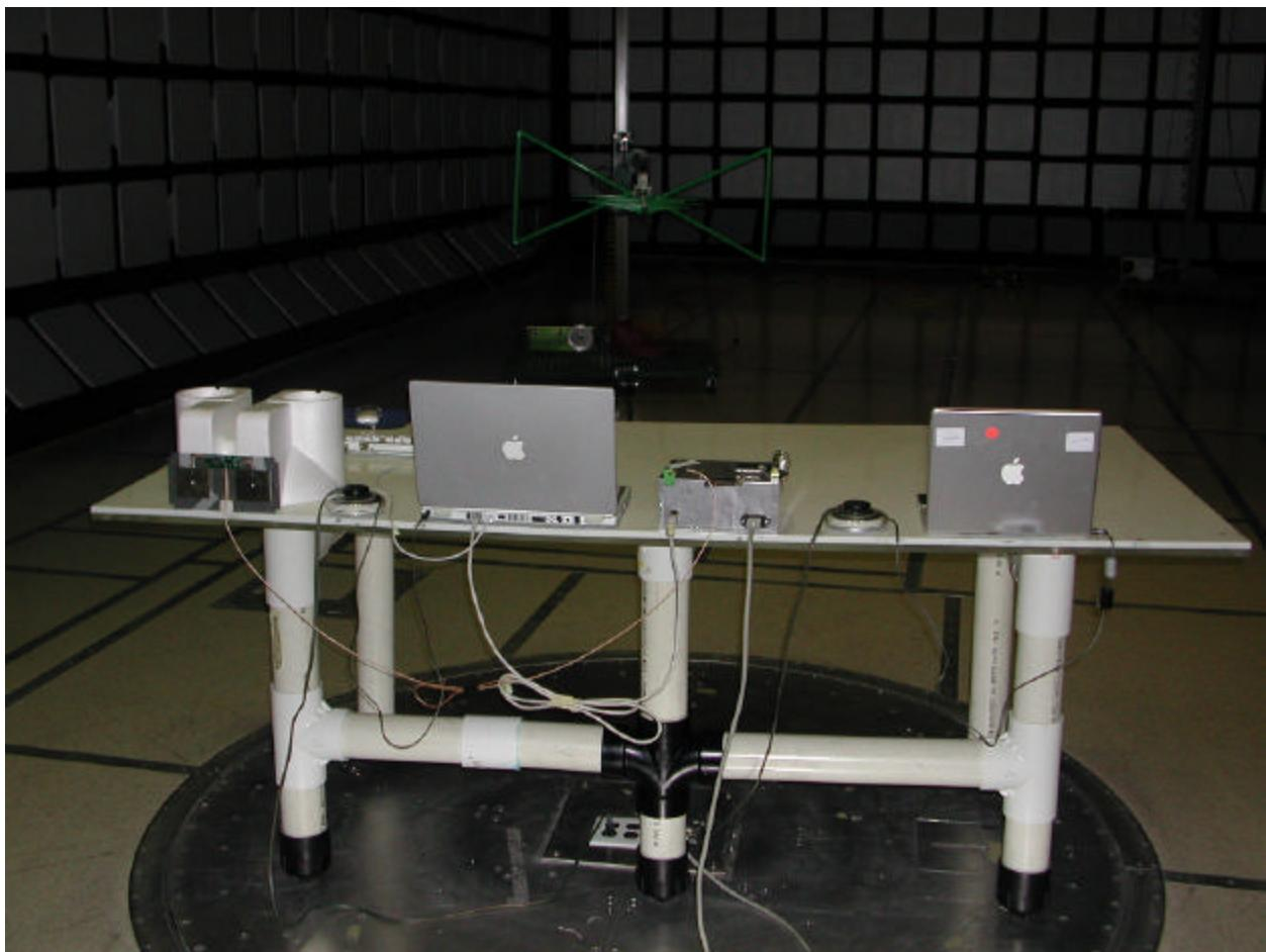
Powerline Conducted Emissions Measurement
