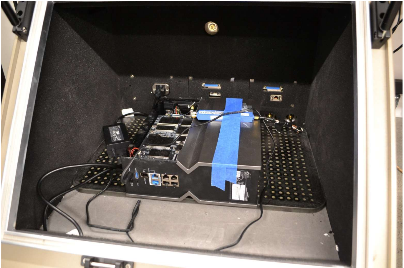
Figure A-5 Wi-Fi Access Point setup in Isolation Box
