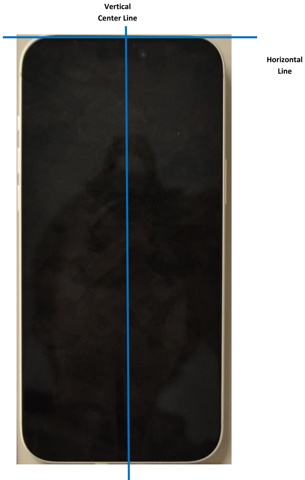
Photograph 5: Handset Vertical and Horizontal Reference Lines
