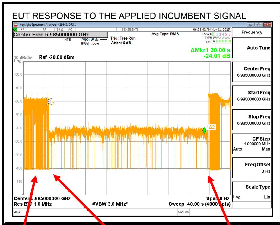
Transmissions cease while the Incumbent AWGN Signal is present and resumes after it is removed. Observed transmissions are a function of the Bandwidth Reduction feature on an adjacent channel.
