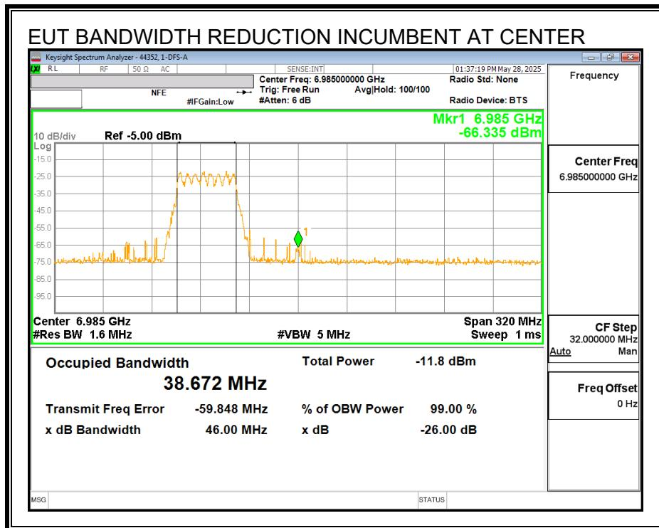
With the Incumbent Signal set to the Center  $f_{c1}$  the EUT continues to operate at a reduced 40MHz nominal bandwidth.
