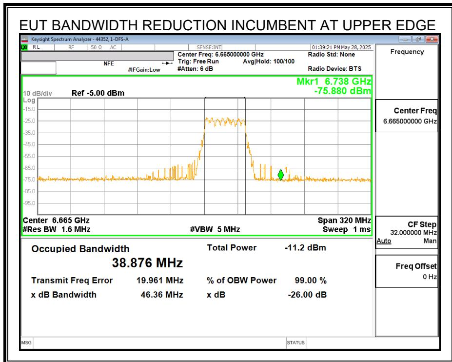
With the Incumbent Signal set to the upper edge  $f_{c3}$  the EUT continues to operate at a reduced 40MHz nominal bandwidth.
