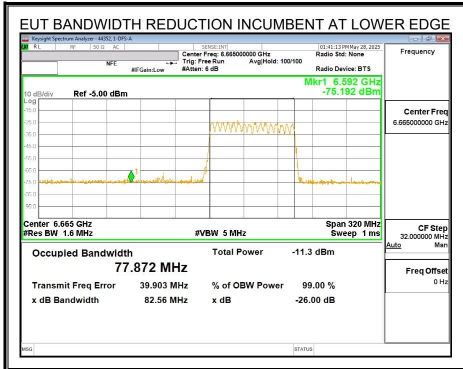
With the Incumbent Signal set to the Lower Edge  $f_{c2}$  the EUT continues to operate at a reduced 80MHz nominal bandwidth.
