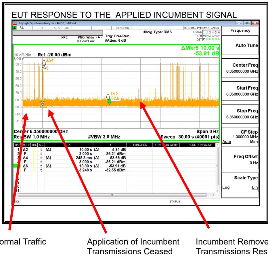
Transmissions cease within 248.3ms while the Incumbent AWGN Signal is present and resume after it is removed.
