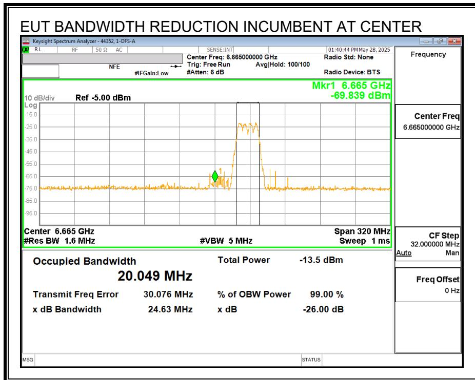
With the Incumbent Signal set to the Center  $f_{c1}$  the EUT continues to operate at a reduced 20MHz nominal bandwidth.
