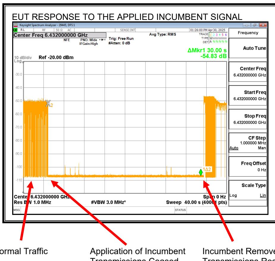
Transmissions cease while the Incumbent AWGN Signal is present and resume after it is removed. Observed transmissions are a function of the Bandwidth Reduction feature on an adjacent channel.
