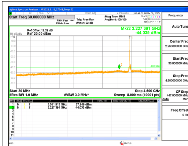
5G NR n48 40MHz QPSK Low Channel RB1-0 (30MHz to 4.5GHz)
