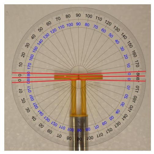
$\bullet~$  The center red line indicates that the arms of the dipole fall within  $\pm 2^{\circ}$
