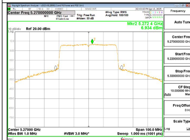
40MHz - Mid Channel – SU (UNII-2A) – ANT 5
