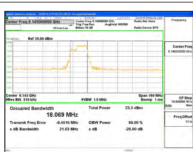
80MHz - Mid Channel – 106+26T RU85 (UNII-5) – ANT 6
