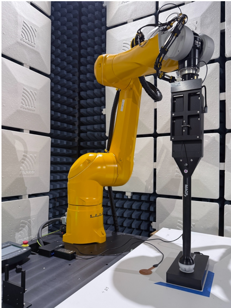
Figure 2: SPEAG DASY8 system with MAGPy V2.0 measurement probe
