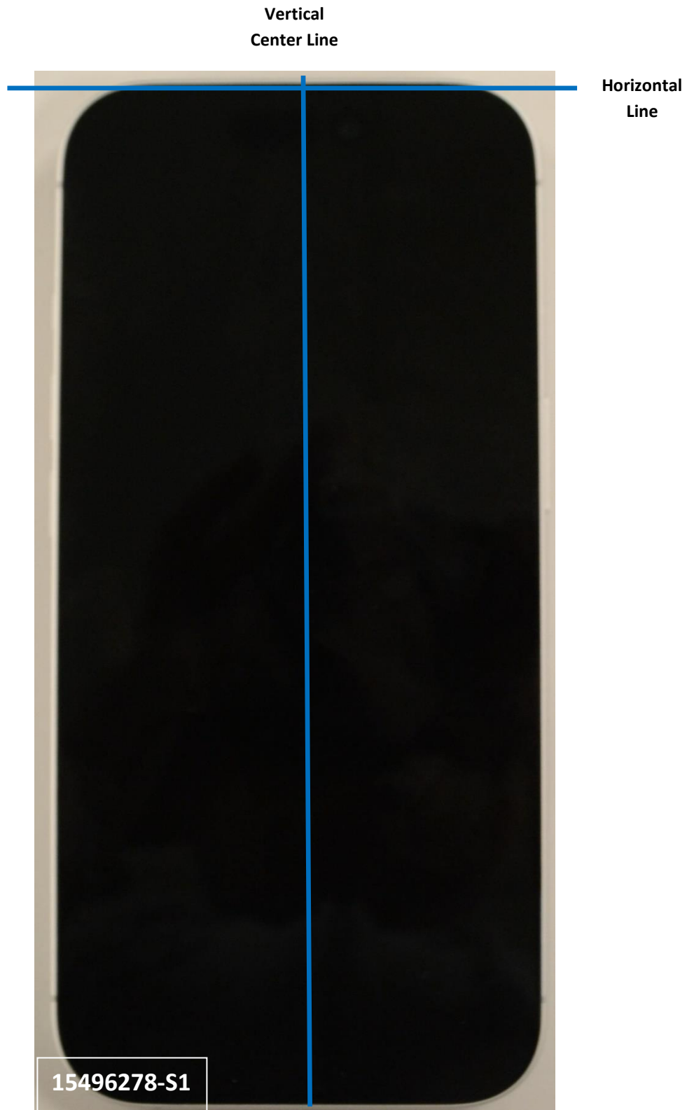
Photograph 4: Handset Vertical and Horizontal Reference Lines
