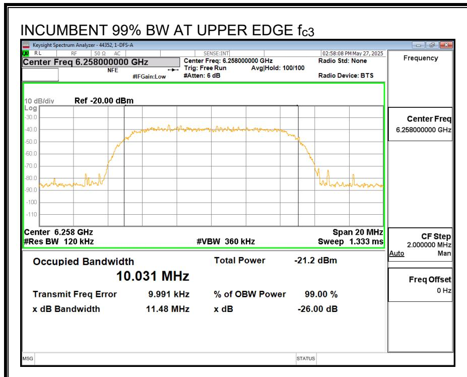
**MINIMUM PASSING INCUMBENT SIGNAL POWER AT TEST FIXTURE**
