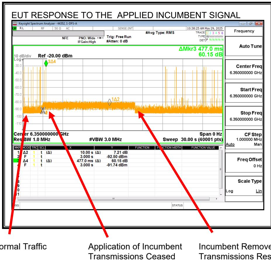
Transmissions cease within 477ms while the Incumbent AWGN Signal is present and resume after it is removed.
