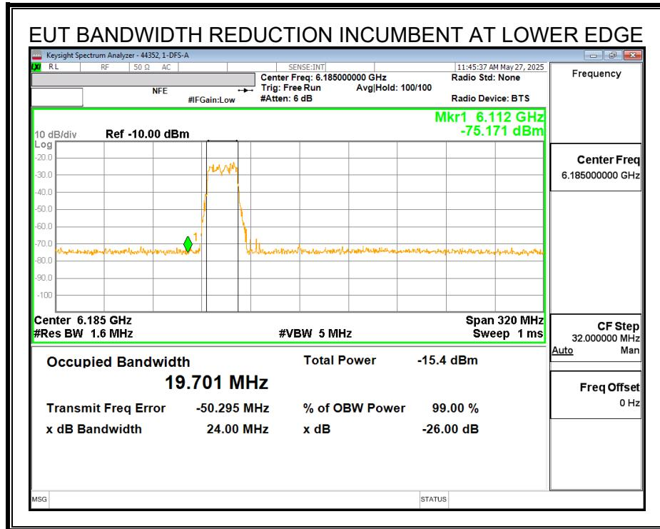
With the Incumbent Signal set to the Lower Edge  $f_{c2}$  the EUT continues to operate at a reduced 20MHz nominal bandwidth.
