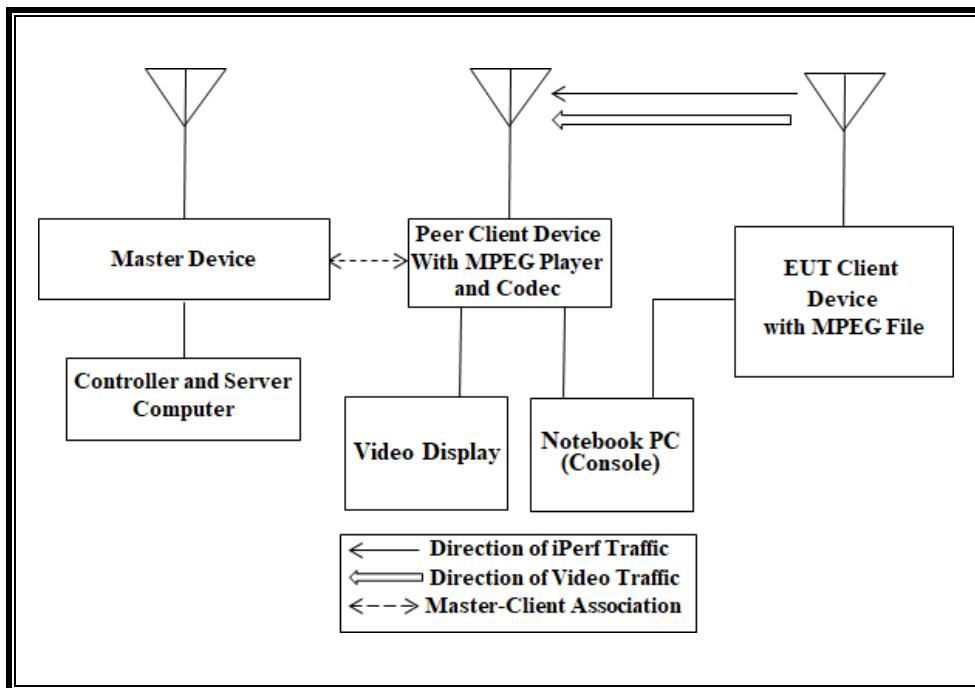
**RADIATED METHOD EUT TEST SETUP WHEN MONITORING THE PEER CLIENT DEVICE)**
