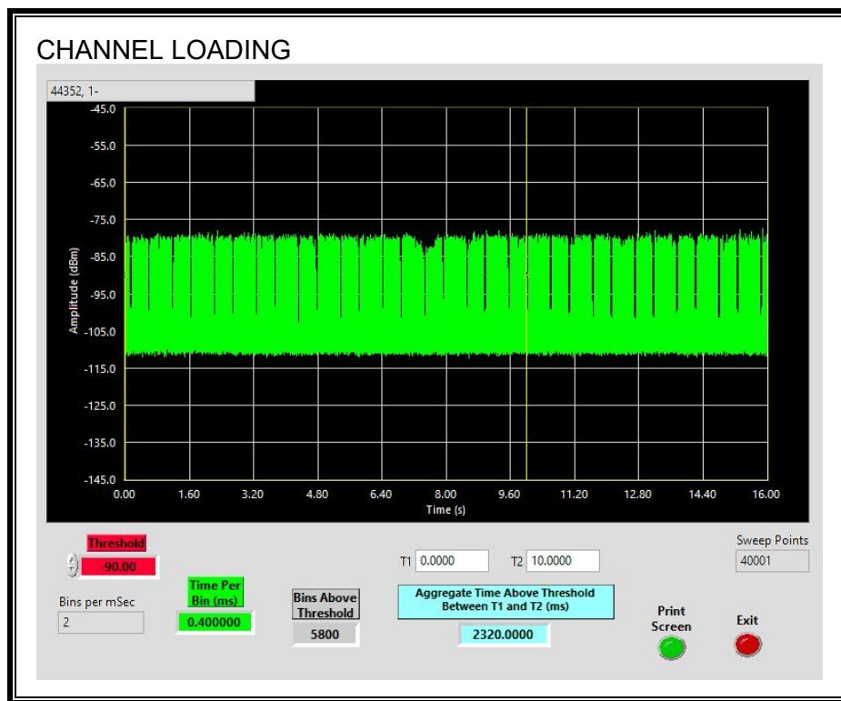
The level of traffic loading on the channel by the EUT is 23.2%
