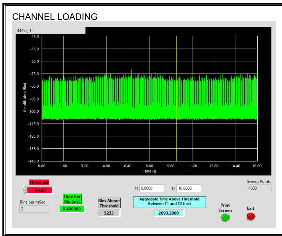
The level of traffic loading on the channel by the EUT is 20.932%
