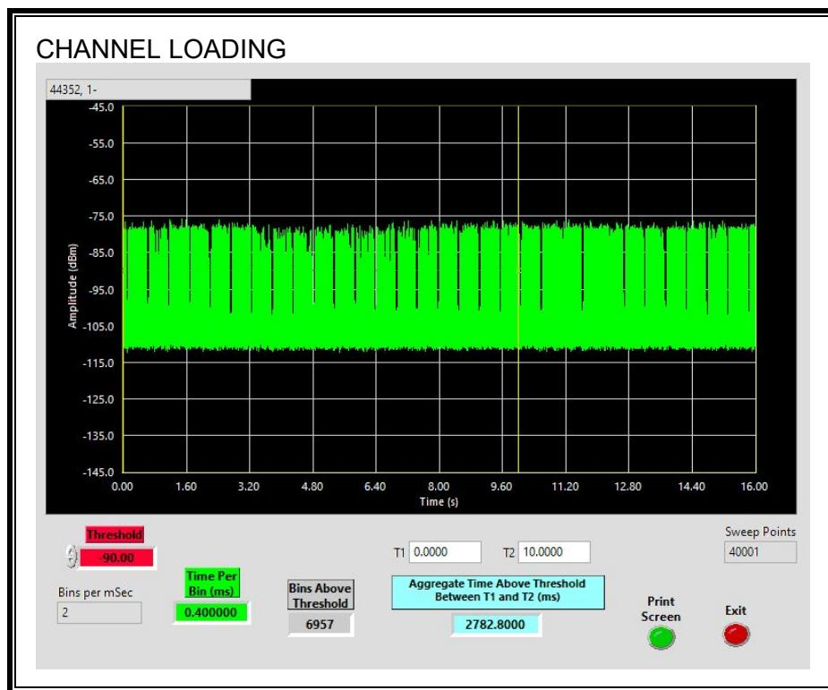
The level of traffic loading on the channel by the EUT is 27.828%
