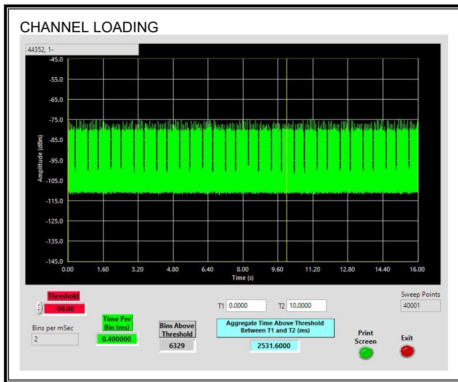
The level of traffic loading on the channel by the Peer Client is 25.316%
