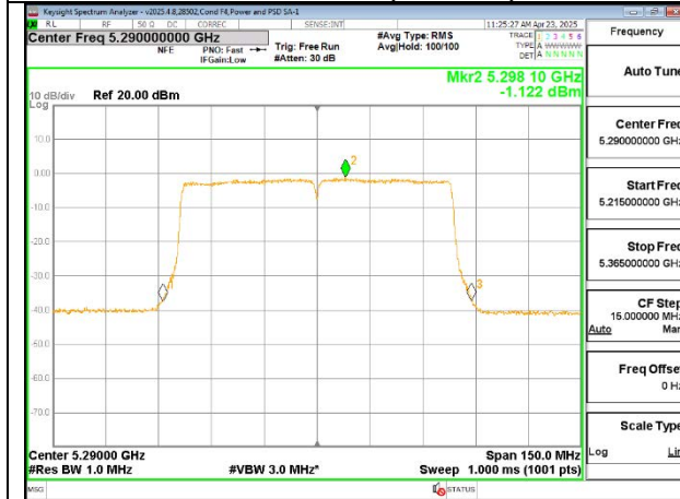
80MHz - Mid Channel (UNII-2A) – ANT 6
