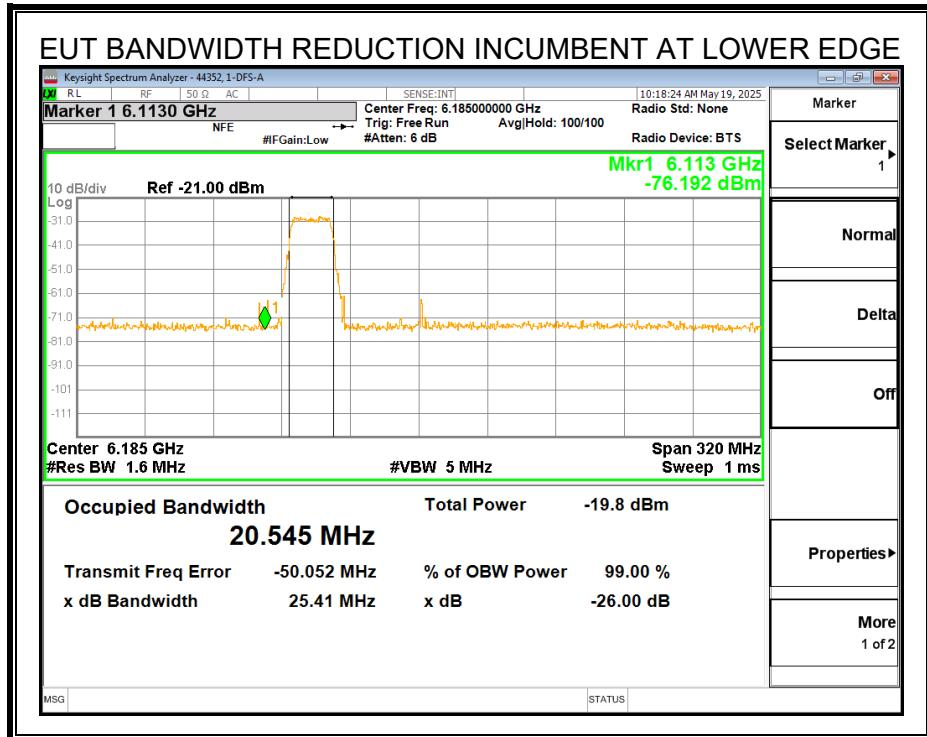
With the Incumbent Signal set to the Lower Edge  $f_{c2}$  the EUT continues to operate at a reduced 20MHz nominal bandwidth.
