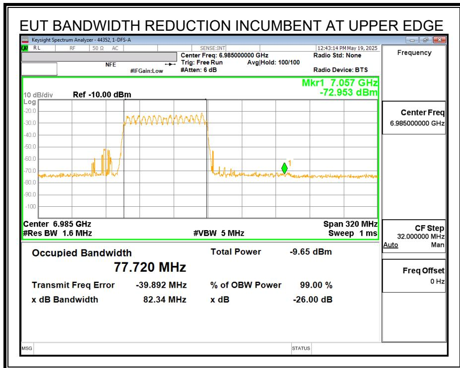
With the Incumbent Signal set to the upper edge  $f_{c3}$  the EUT continues to operate at a reduced 80MHz nominal bandwidth.
