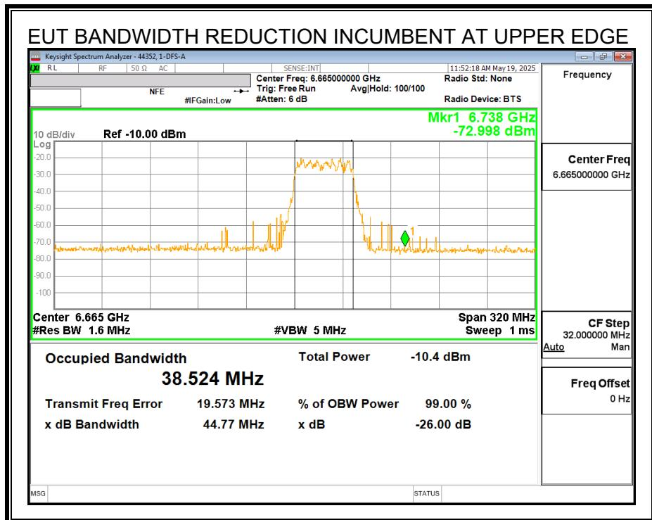
With the Incumbent Signal set to the upper edge  $f_{c3}$  the EUT continues to operate at a reduced 40MHz nominal bandwidth.
