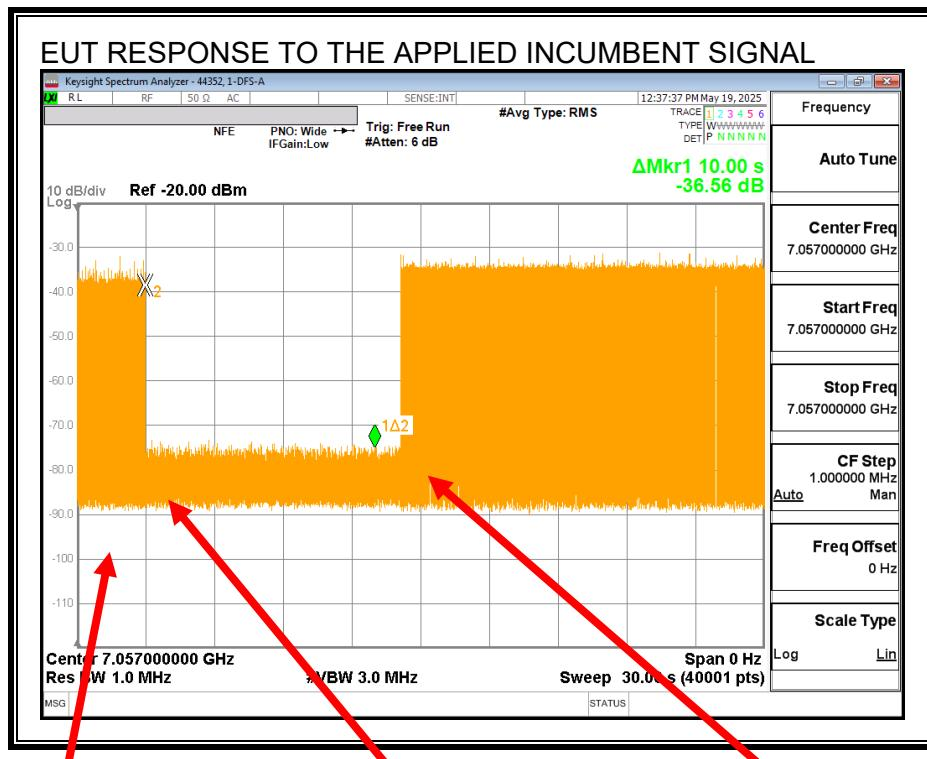
Transmissions cease on the incumbered channel while the Incumbent AWGN Signal is present with the bandwidth reducing from 160 MHz to 80 MHz on an adjacent and resume after it is removed.
