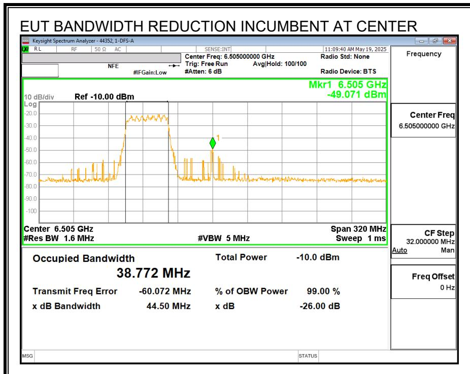
With the Incumbent Signal set to the Center  $f_{c1}$  the EUT continues to operate at a reduced 40MHz nominal bandwidth.
