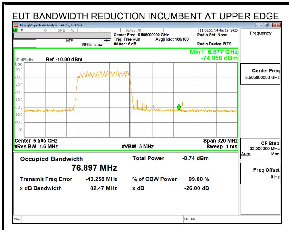
With the Incumbent Signal set to the upper edge  $f_{c3}$  the EUT continues to operate at a reduced 80MHz nominal bandwidth.
