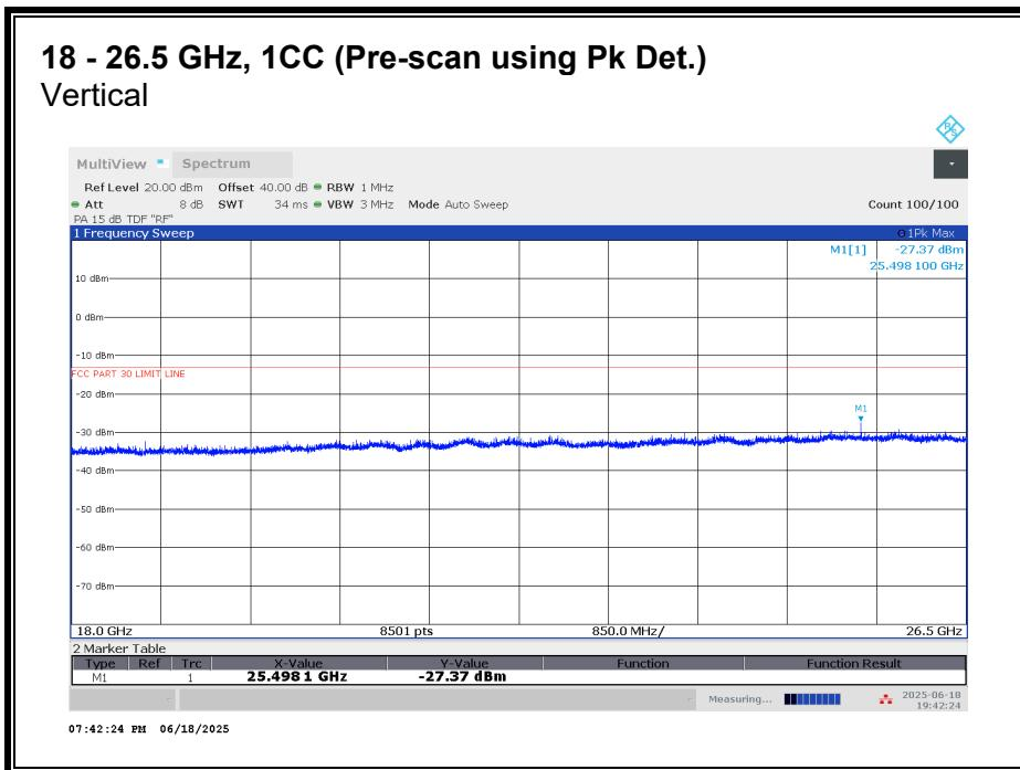
Emissions detected using Peak Detection at pre-scan. Avg EIRP or TRP was measured.
