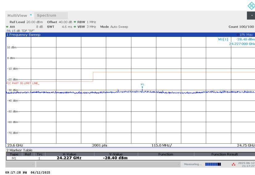
Emission detected using Peak Detection at pre-scan. Avg EIRP or TRP was measured.
