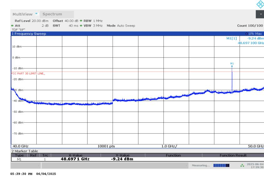
Emissions detected using Peak Detection at pre-scan. Avg EIRP or TRP was measured.
