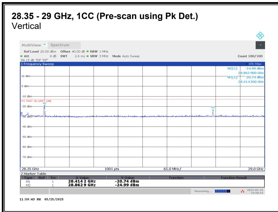
Emissions detected using Peak Detection at pre-scan. Avg EIRP or TRP was measured.
