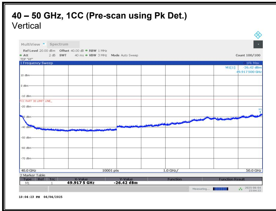
No emission detected using Peak Detection.
