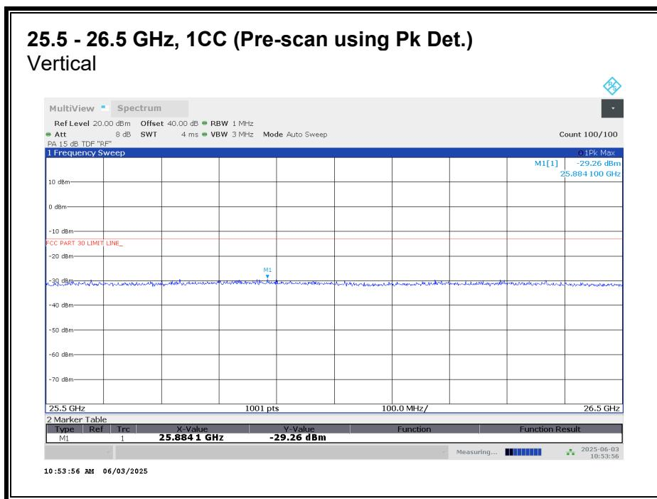
No emission detected using Peak Detection.
