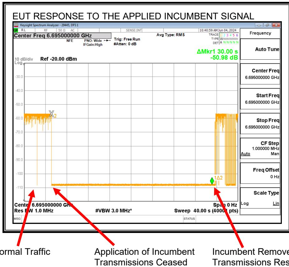
Transmissions cease while the Incumbent AWGN Signal is present and resume after it is removed.
