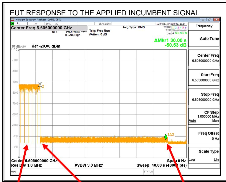
Transmissions cease while the Incumbent AWGN Signal is present and resume after it is removed.
