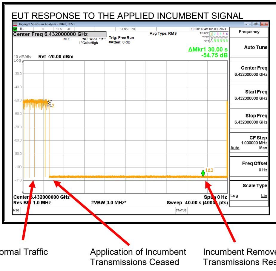
Transmissions cease while the Incumbent AWGN Signal is present and resume after it is removed.
