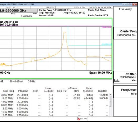
LTE B25 3MHz QPSK High Channel RB1-14
