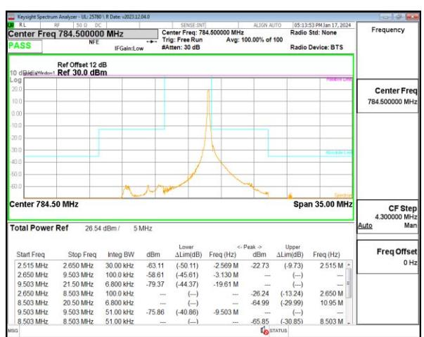
LTE B13 5MHz QPSK Low Channel RB1-24
