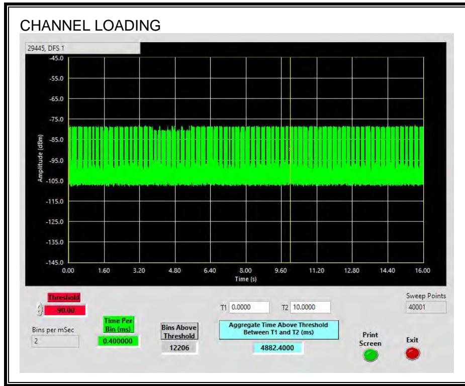
The level of traffic loading on the channel by the EUT is 48.82%
