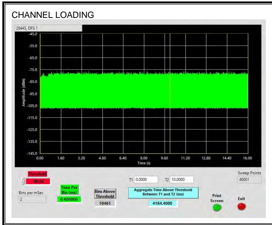
The level of traffic loading on the channel by the EUT is 41.84%
