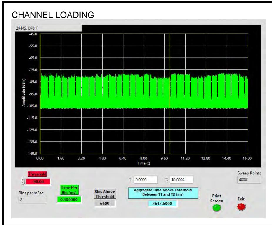
The level of traffic loading on the channel by the EUT is 26.43%
