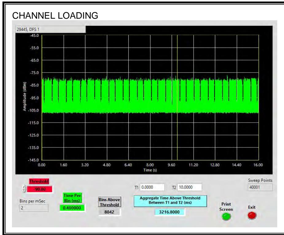
The level of traffic loading on the channel by the EUT is 32.16%
