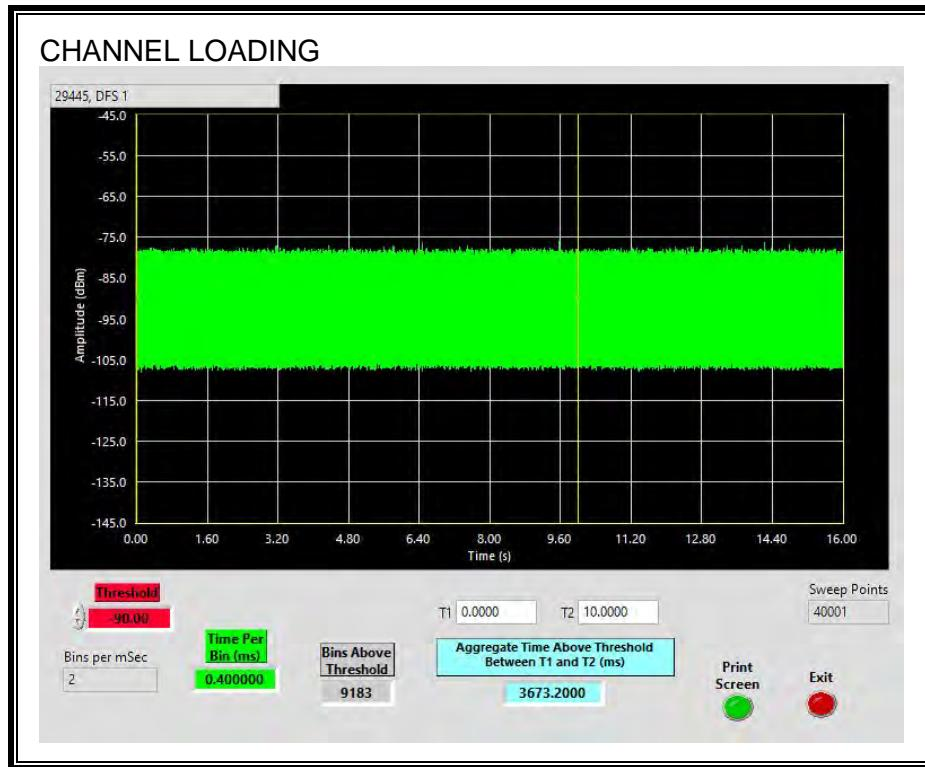
The level of traffic loading on the channel by the EUT is 36.73%
