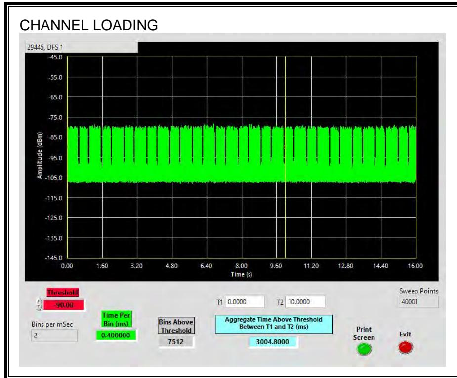
The level of traffic loading on the channel by the EUT is 30.04%
