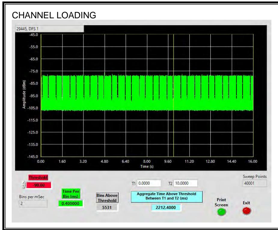
The level of traffic loading on the channel by the Peer Slave is 22.12%
