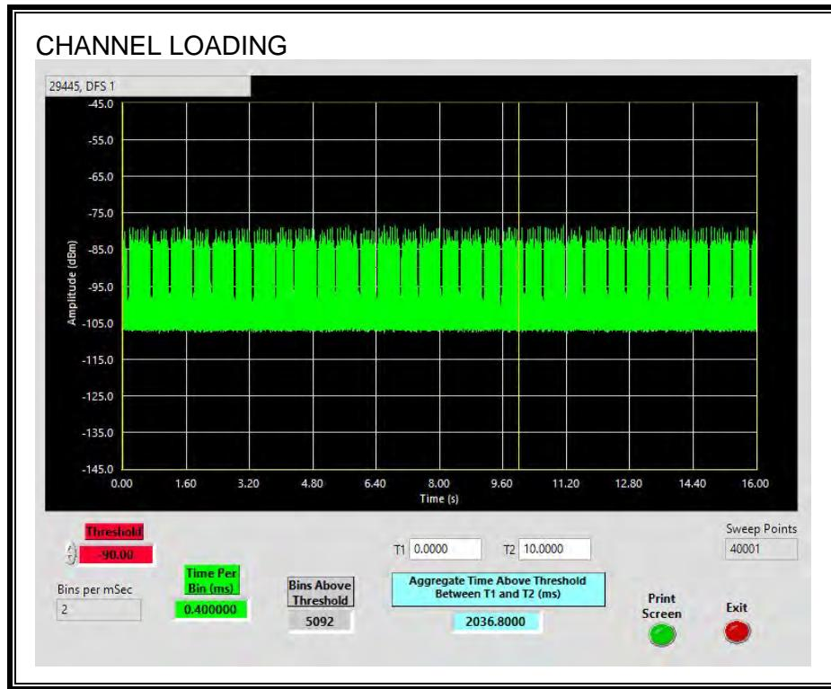
The level of traffic loading on the channel by the Peer Slave is 20.36%
