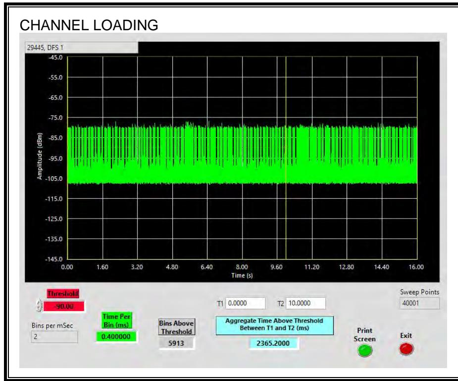
The level of traffic loading on the channel by the EUT is 23.65%
