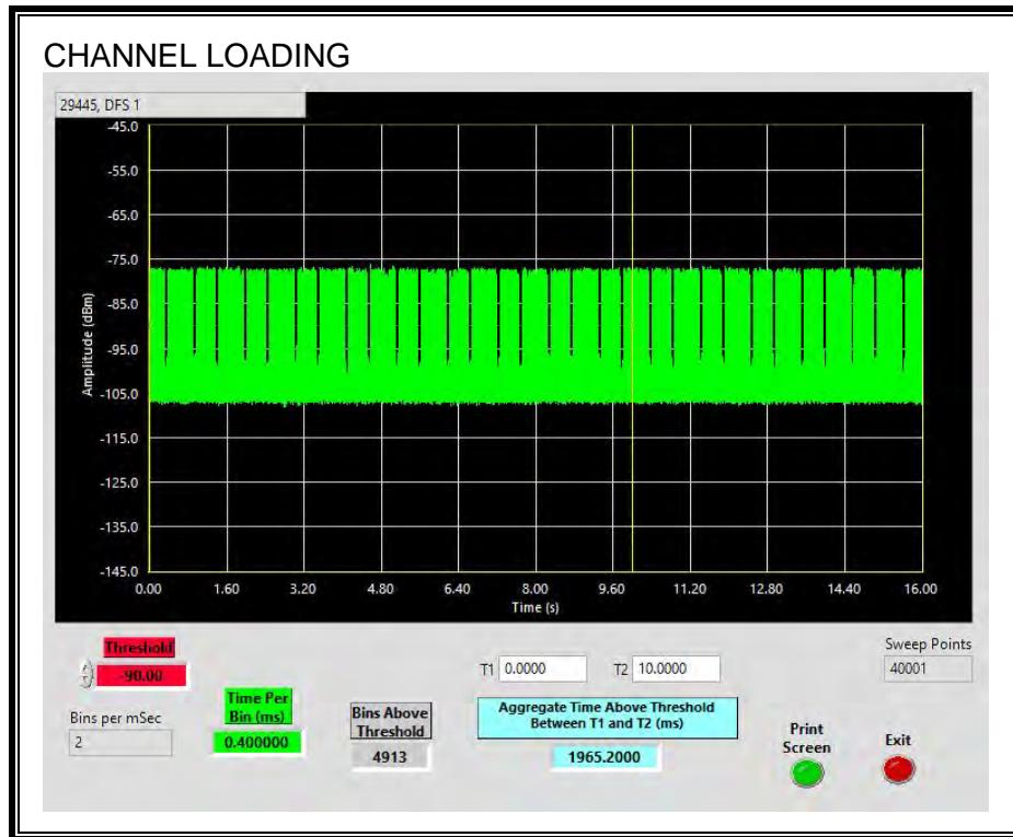
The level of traffic loading on the channel by the Peer Slave is 19.65%
