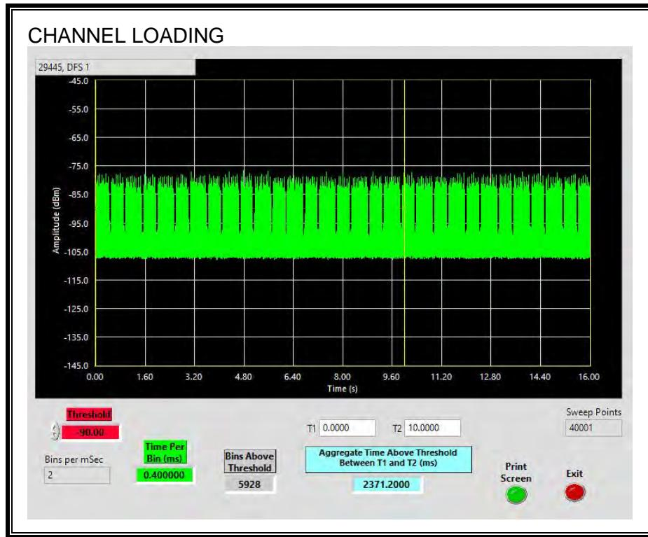
The level of traffic loading on the channel by the EUT is 23.71%
