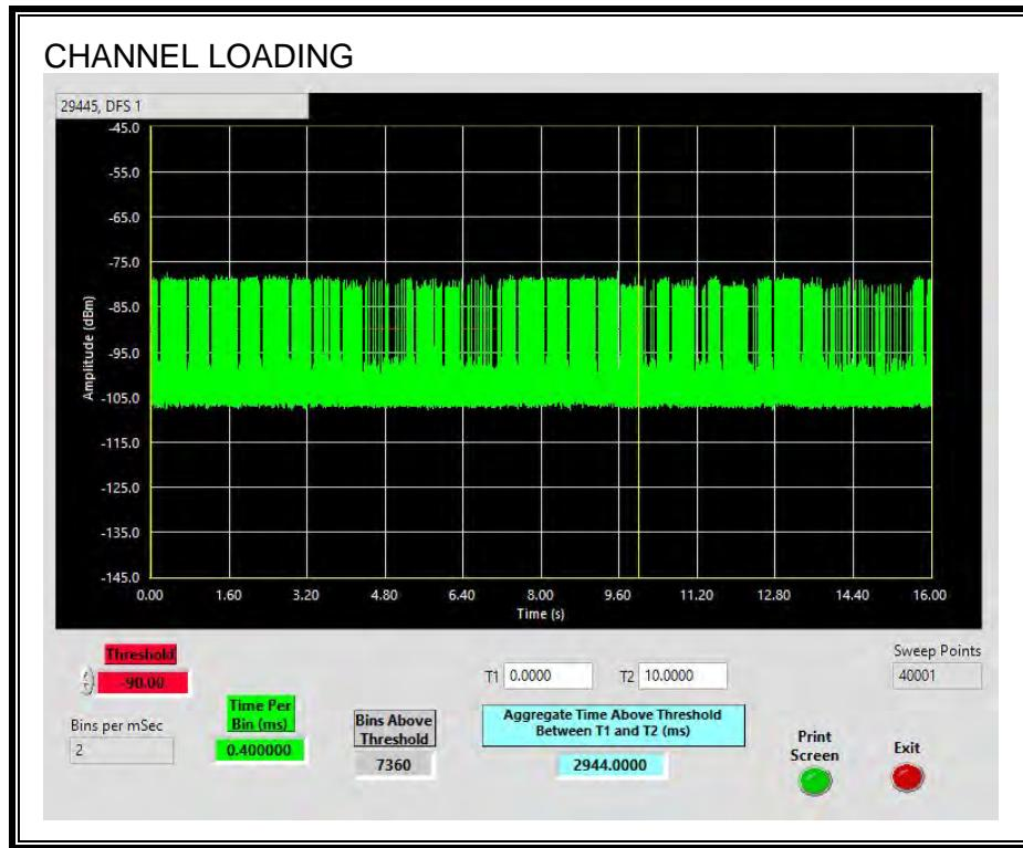
The level of traffic loading on the channel by the EUT is 29.44%
