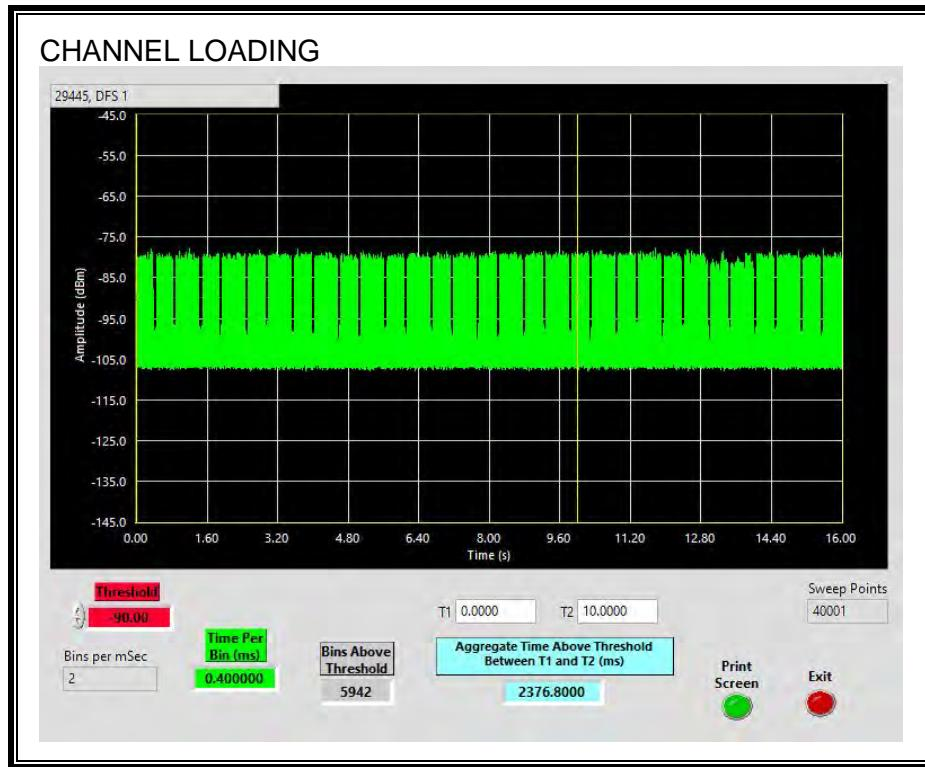
The level of traffic loading on the channel by the EUT is 23.76%
