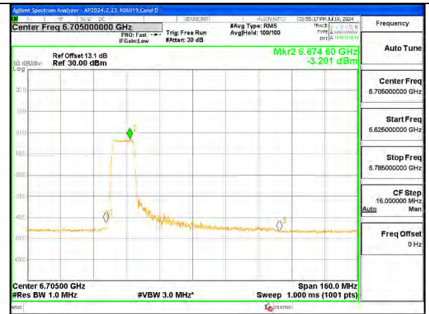
80MHz - Mid Channel – MRU106+26T-RU82 (UNII-7) – Ant 1
