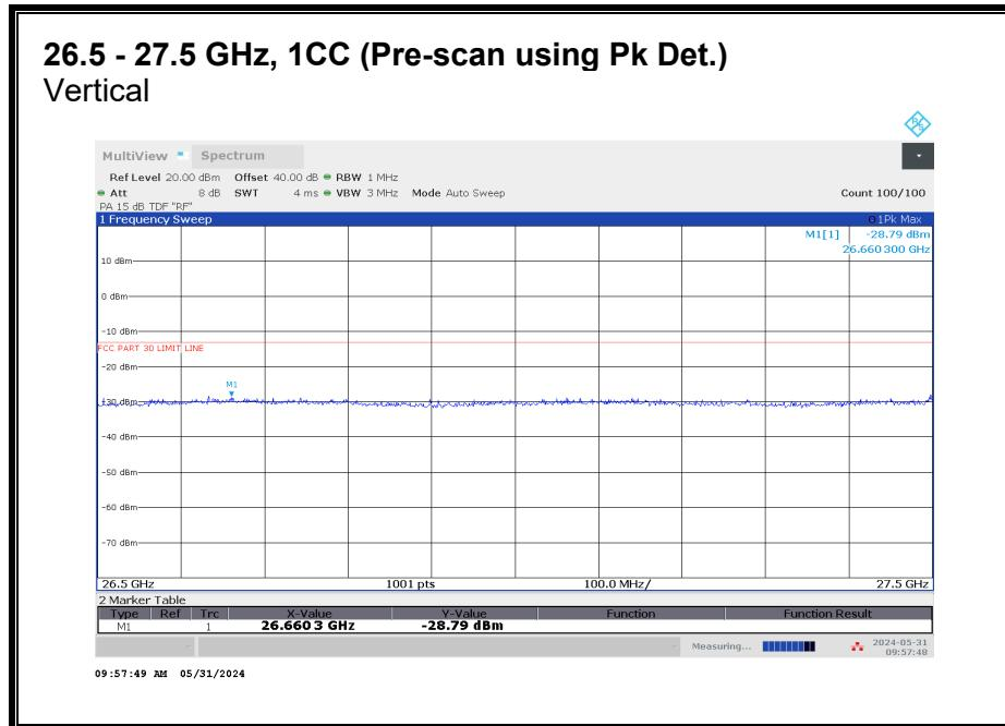
No emission detected using Peak Detection.
