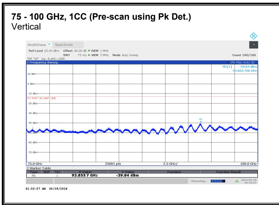
No emission detected using Peak Detection.
