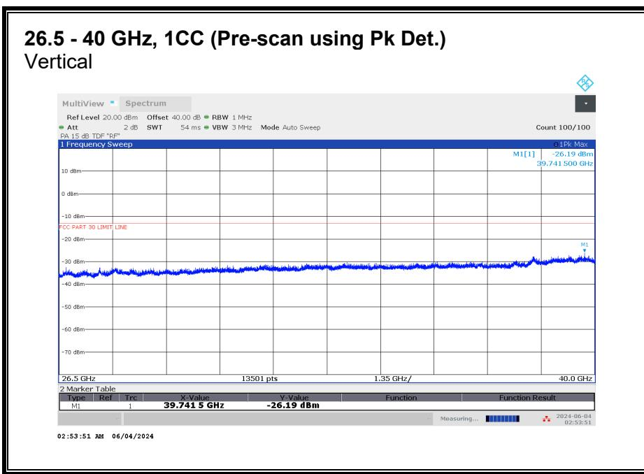
No emission detected using Peak Detection.
