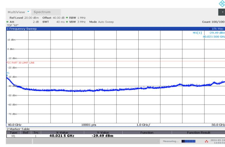
No emission detected using Peak Detection.
