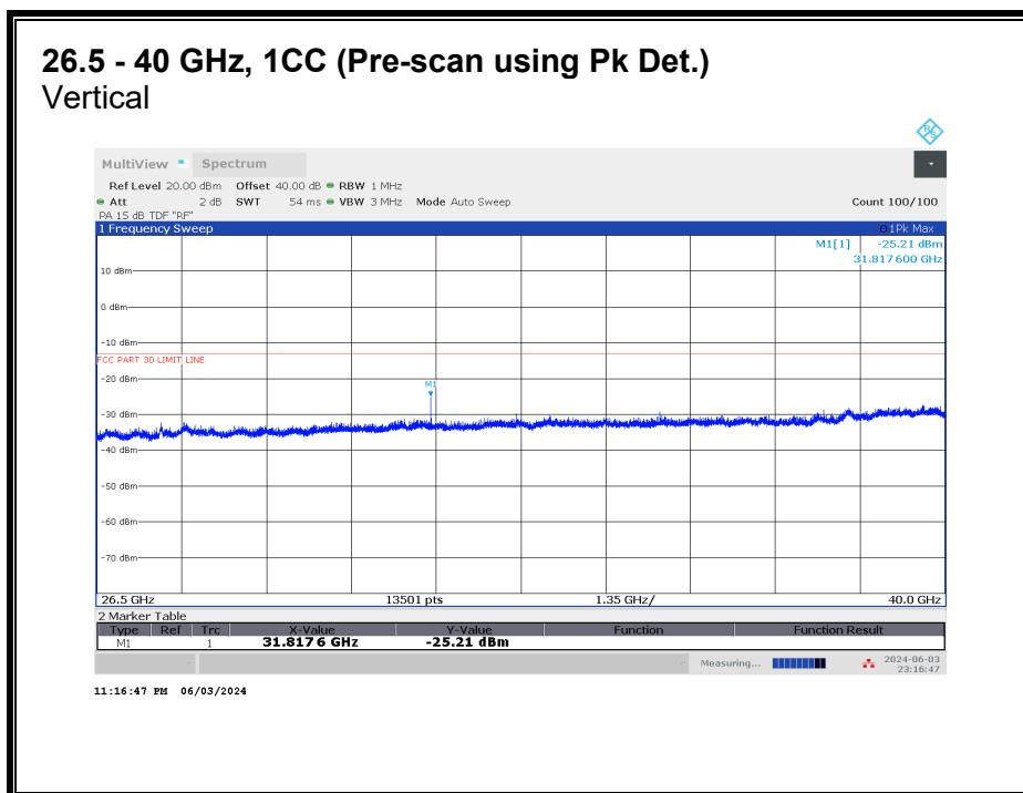
Emissions detected using Peak Detection at pre-scan. Avg EIRP was measured.
