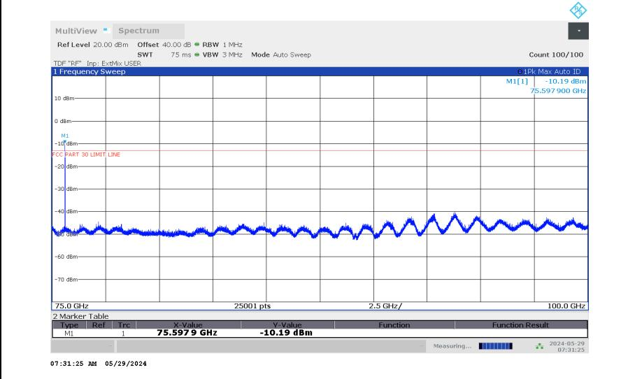
Emissions detected using Peak Detection at pre-scan. Avg EIRP was measured.
