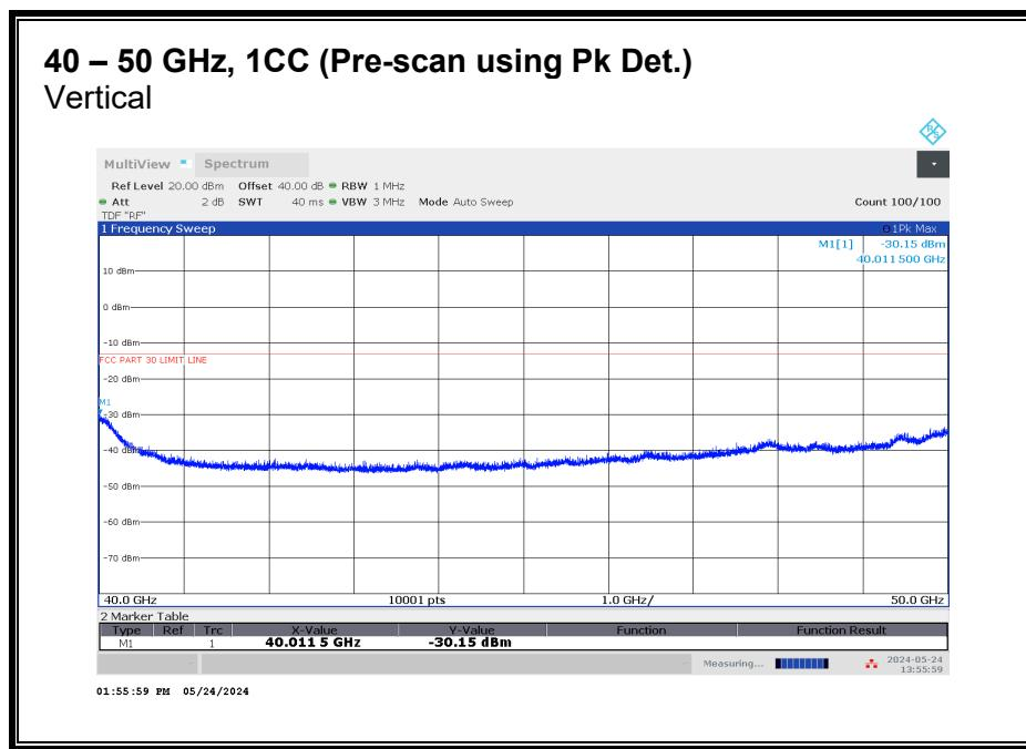
No emission detected using Peak Detection.
