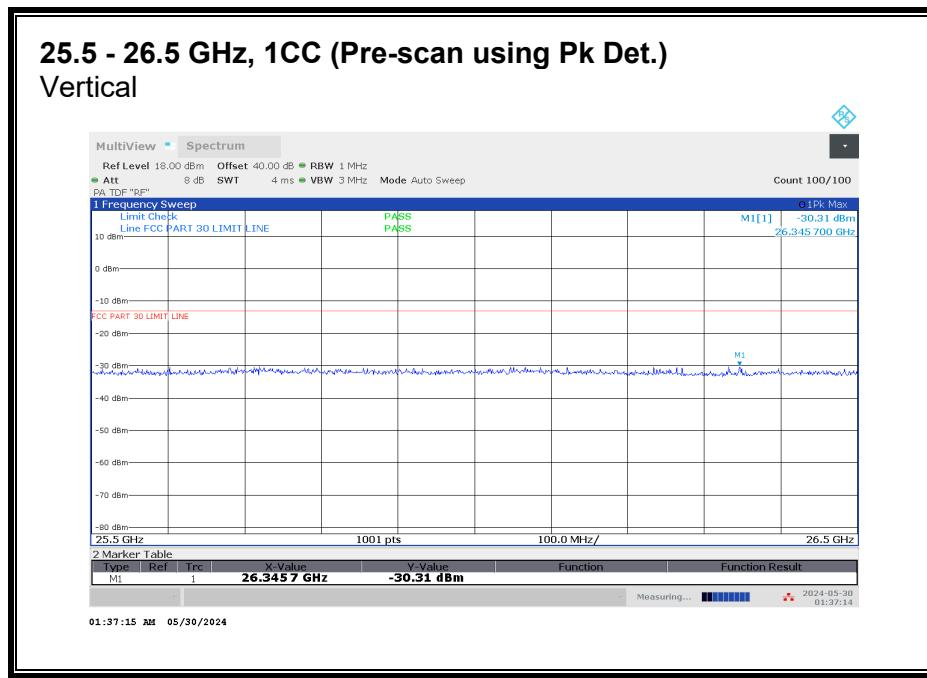
No emission detected using Peak Detection.
