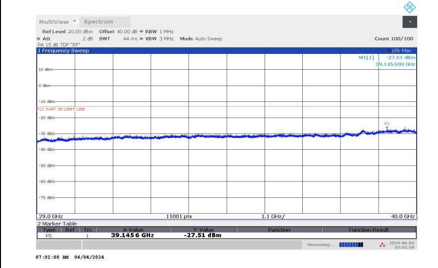
Emission detected using Peak Detection at pre-scan. Avg EIRP was measured.
