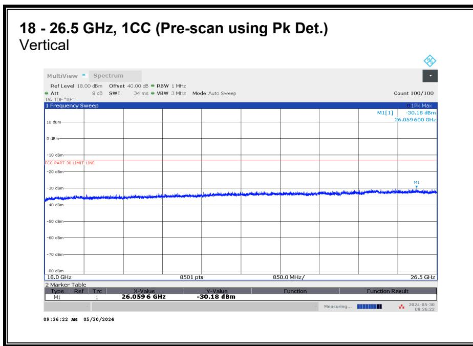
No emission detected using Peak Detection.
