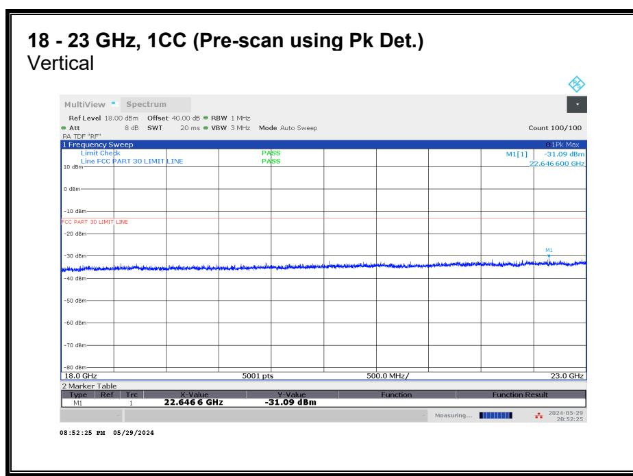
No emission detected using Peak Detection.
