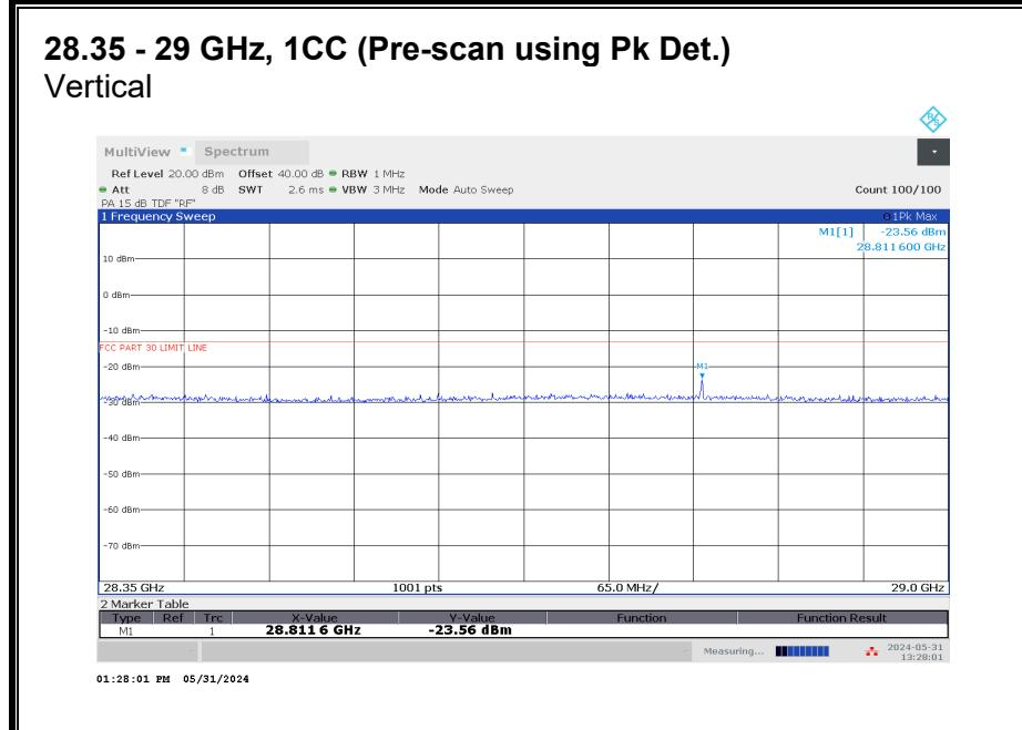
Emissions detected using Peak Detection at pre-scan. Avg EIRP was measured.
