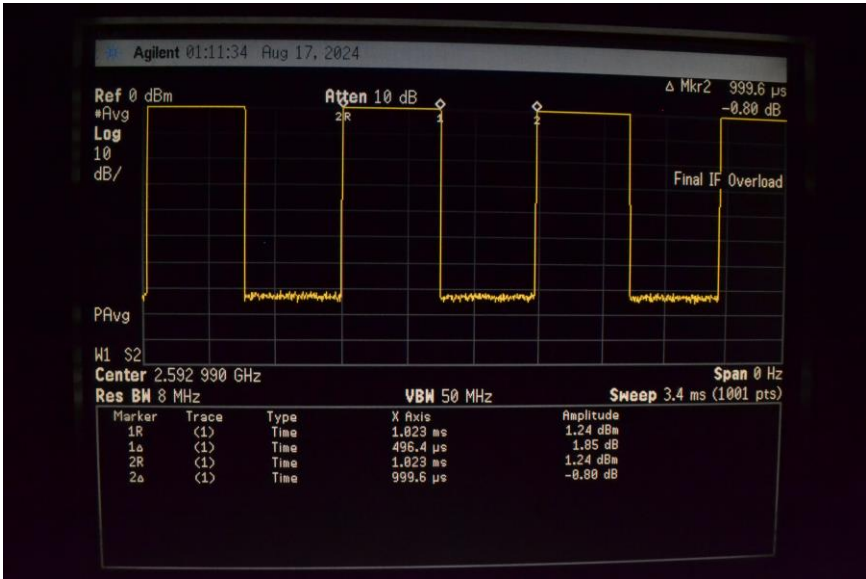
Figure 4: 5G NR TDD Power Class 2, 50% RB
