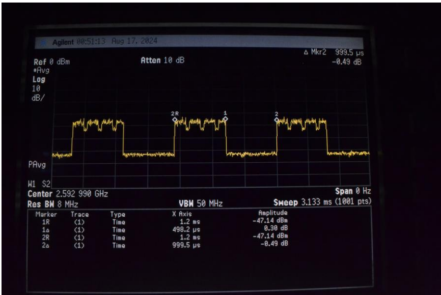
Figure 4: 5G NR TDD Power Class 2, 50% RB
