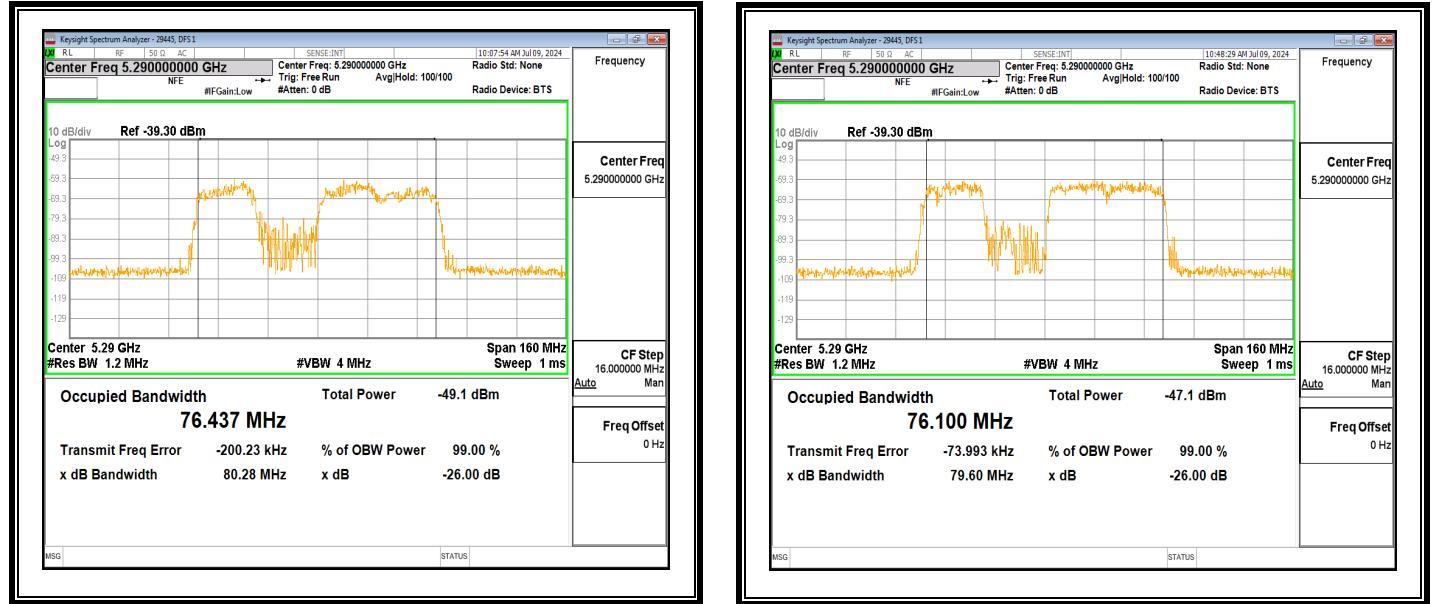
After the puncture command the same 20 MHz Sub-Channel centered at 5260 MHz is disabled by both AP and Client Device.
