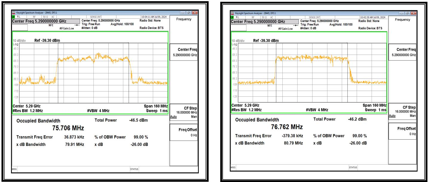
After the puncture command the same 20 MHz Sub-Channel centered at 5280 MHz is disabled by both AP and Client Device.
