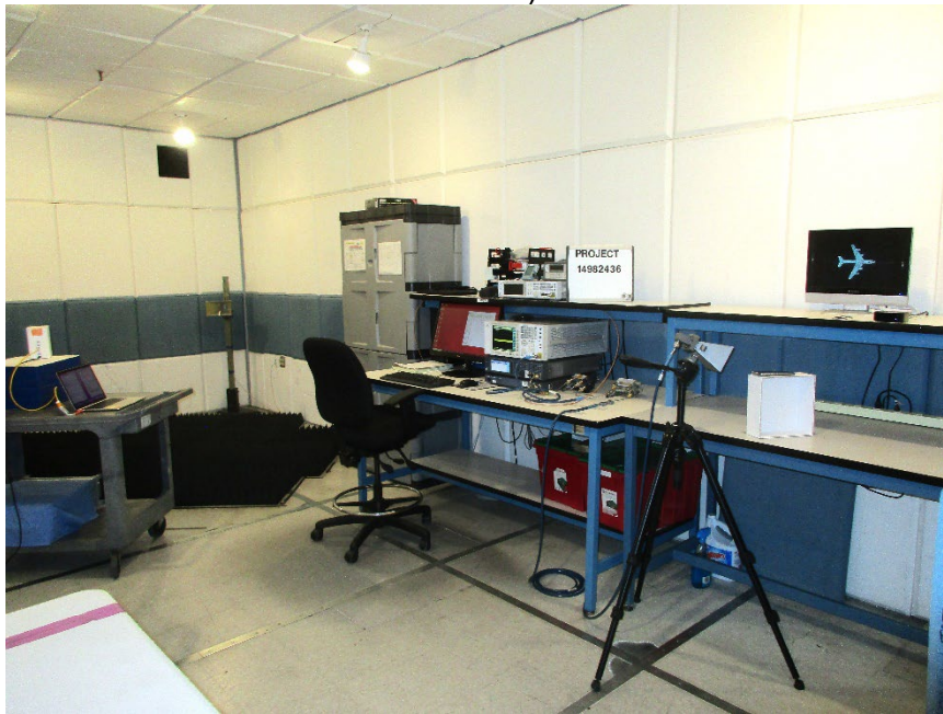
DFS FULL SETUP PHOTO (CLIENT-TO-CLIENT COMMUNICATIONS MODE SETUP)
