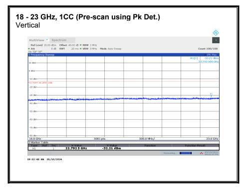
No emission detected using Peak Detection.
