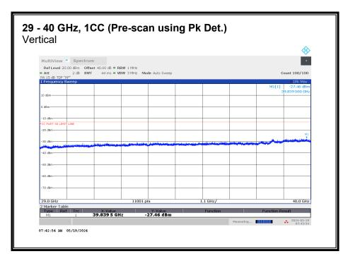
No emission detected using Peak Detection.
