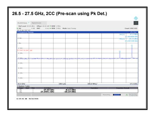
Worst case configuration: SISO-DUAL QPSK (100 MHz + 100 MHz) Low CH RB Offset 1/32 (1RB-M)
