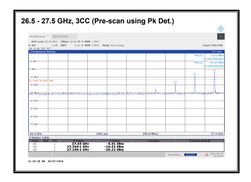
Worst case configuration: SISO-DUAL QPSK (100 MHz + 100 MHz+ 100 MHz) Low CH RB Offset 1/32 (1RB-M)
