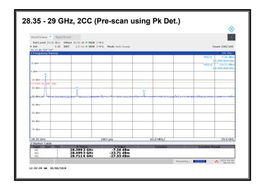
Worst case configuration: SISO-DUAL\_QPSK\_(100 MHz + 100 MHz)\_High CH\_RB Offset 1/32 (1RB-M)
