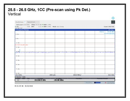
No emission detected using Peak Detection.
