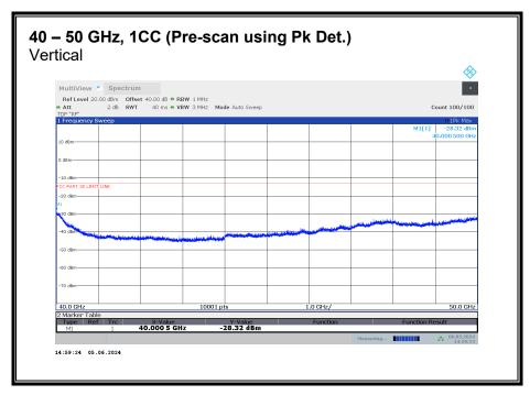
No emission detected using Peak Detection.
