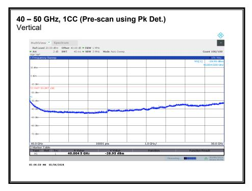
No emission detected using Peak Detection.
