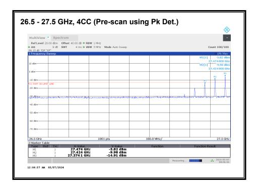
Worst case configuration: SISO-DUAL QPSK (50 MHz + 50 MHz+ 50 MHz+ 50 MHz) Low CH RB Offset 1/15 (1RB-M)
