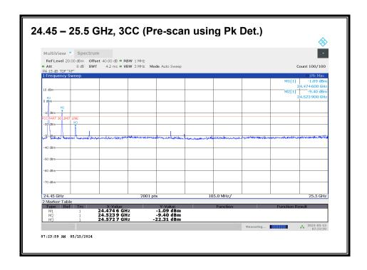
Worst case configuration: SISO-DUAL\_QPSK\_(50 MHz + 50 MHz + 50 MHz)\_High CH\_RB Offset 1/15 (1RB-M)
