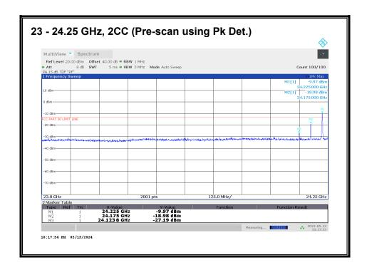
Worst case configuration: SISO-DUAL\_QPSK\_(50 MHz + 50 MHz)\_Low CH\_RB Offset 1/15 (1RB-M)
