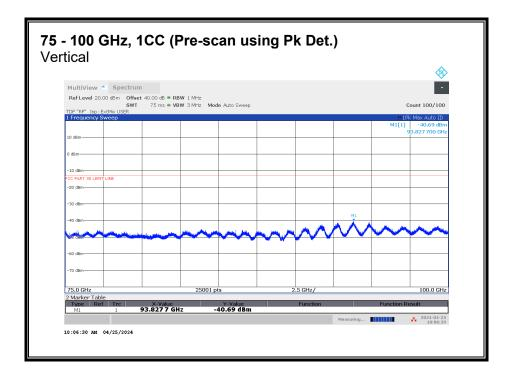
No emission detected using Peak Detection.
