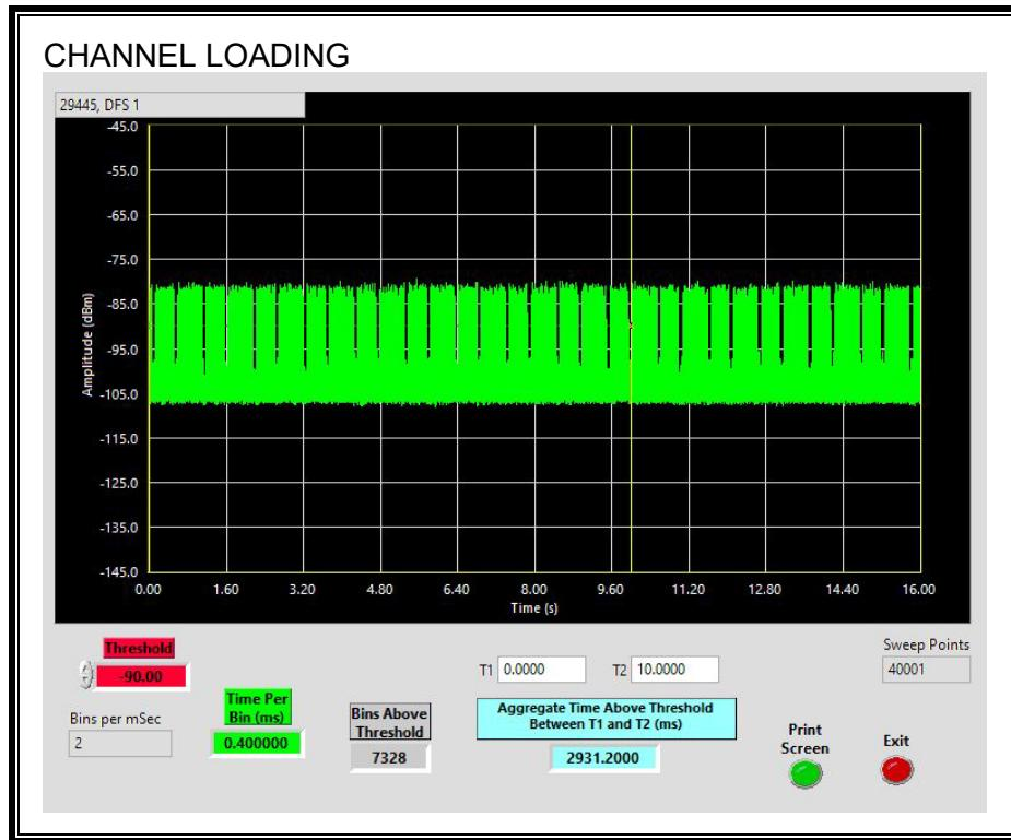
The level of traffic loading on the channel by the EUT is 29.31%
