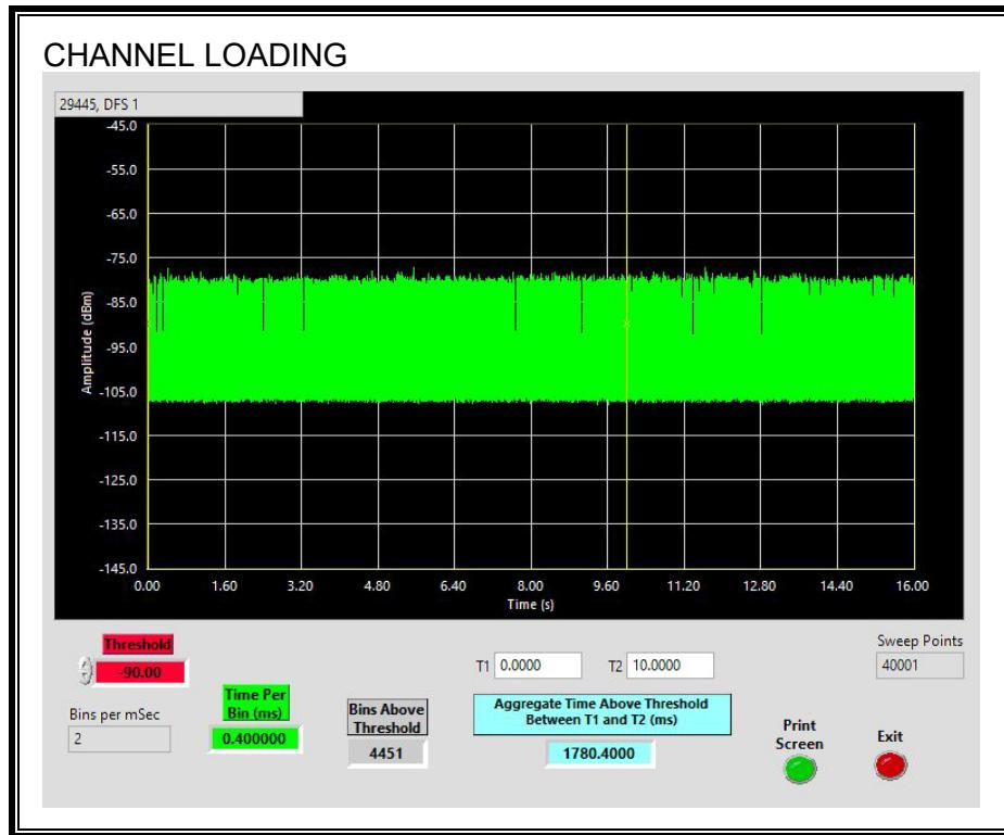
The level of traffic loading on the channel by the EUT is 17.8%
