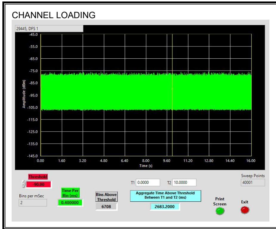
The level of traffic loading on the channel by the EUT is 26.83%
