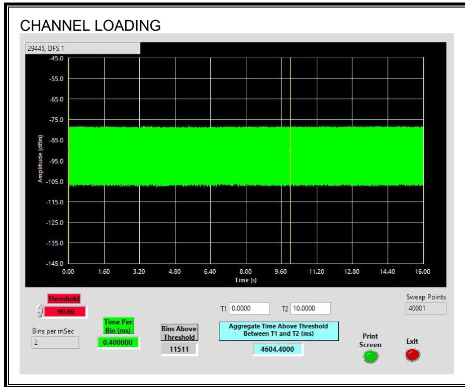
The level of traffic loading on the channel by the EUT is 46.04%
