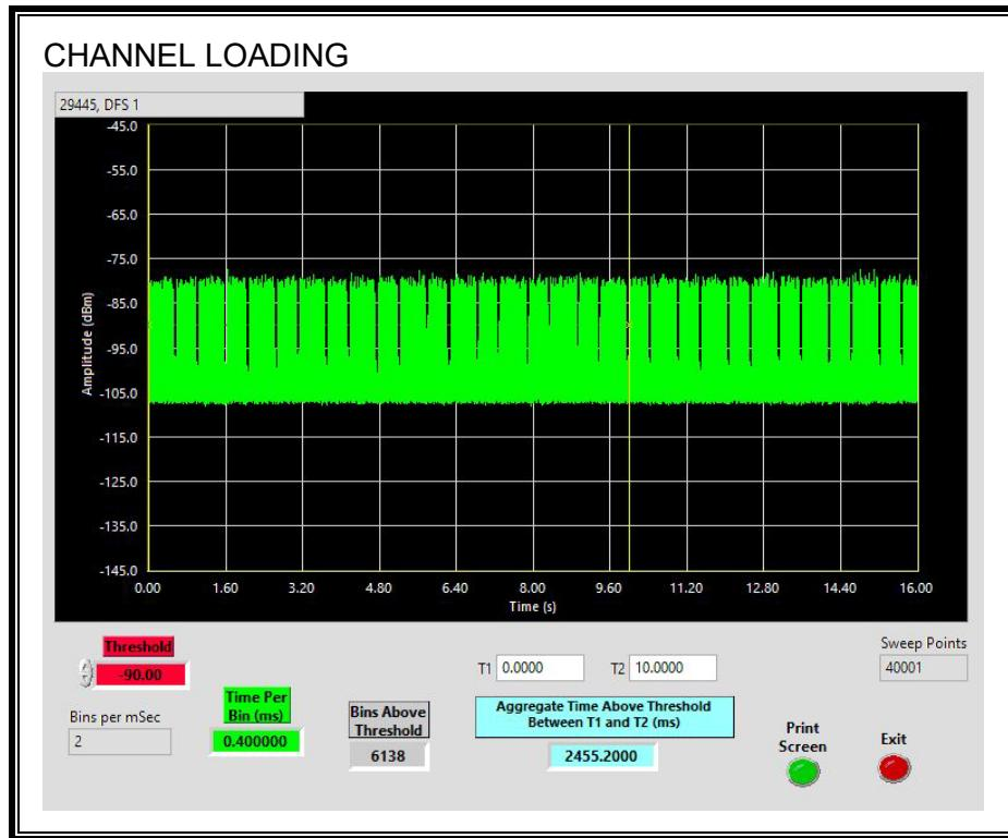
The level of traffic loading on the channel by the EUT is 24.55%
