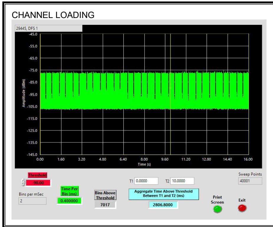
The level of traffic loading on the channel by the EUT is 28.06%
