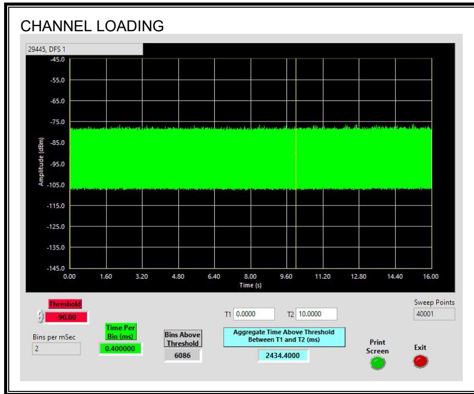
The level of traffic loading on the channel by the EUT is 24.34%
