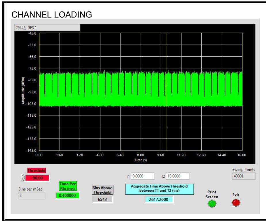
The level of traffic loading on the channel by the EUT is 26.17%
