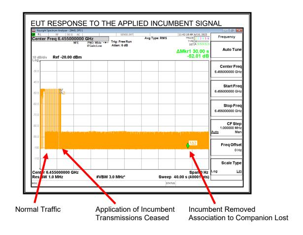
Transmissions cease while the Incumbent AWGN Signal is present and do not resume after it is removed due to the loss of the association to the Companion Device.
