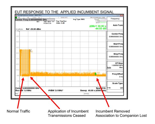
Transmissions cease while the Incumbent AWGN Signal is present and do not resume after it is removed due to the loss of the association to the Companion Device.
