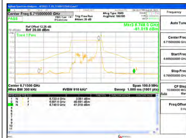
MID CHANNEL Antenna 6
