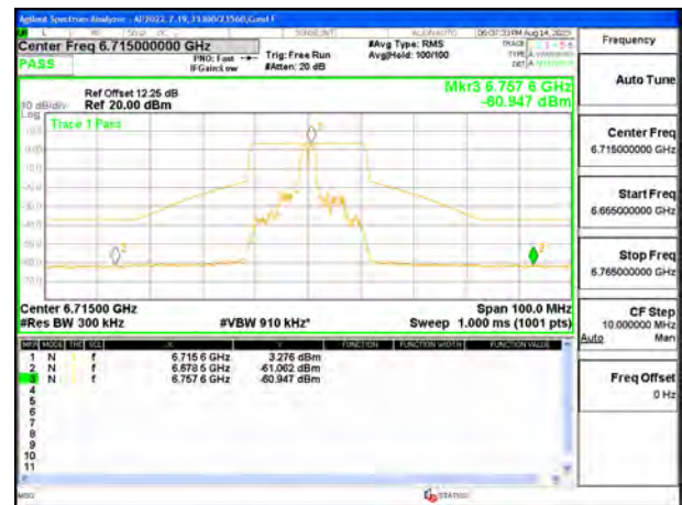
MID CHANNEL Antenna 5
