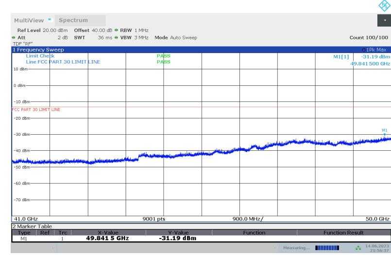
No emission detected using Peak Detection.
