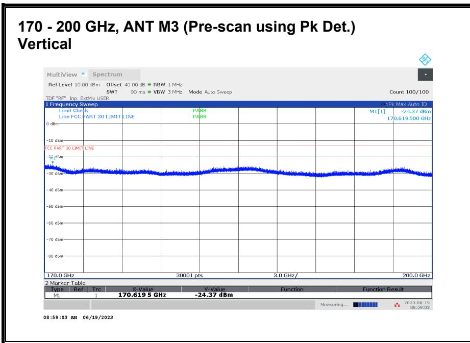
No emission detected using Peak Detection.
