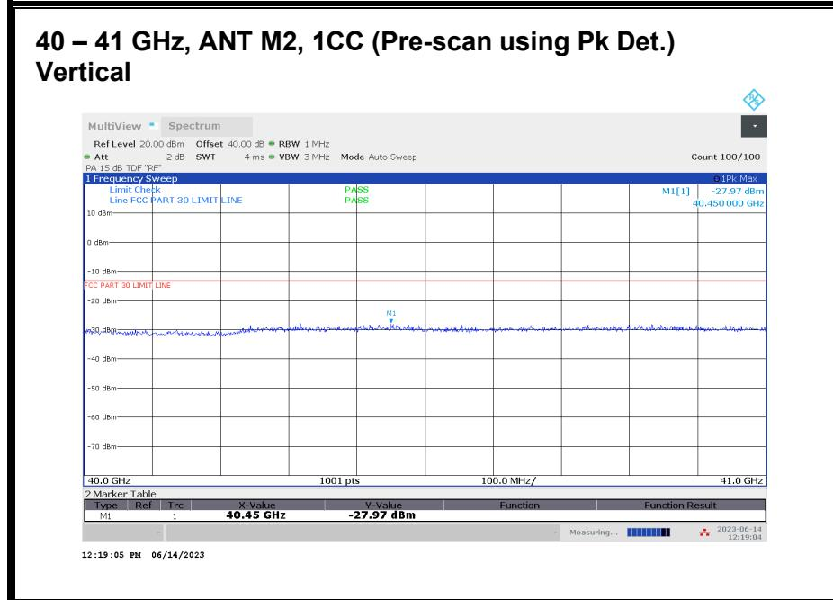
No emission detected using Peak Detection.
