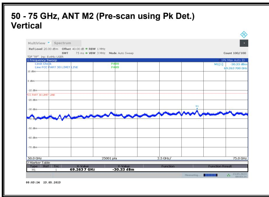
No emission detected using Peak Detection.
