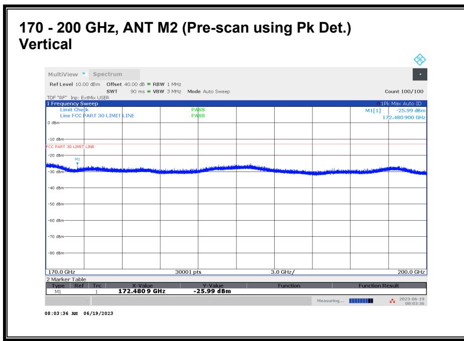
No emission detected using Peak Detection.
