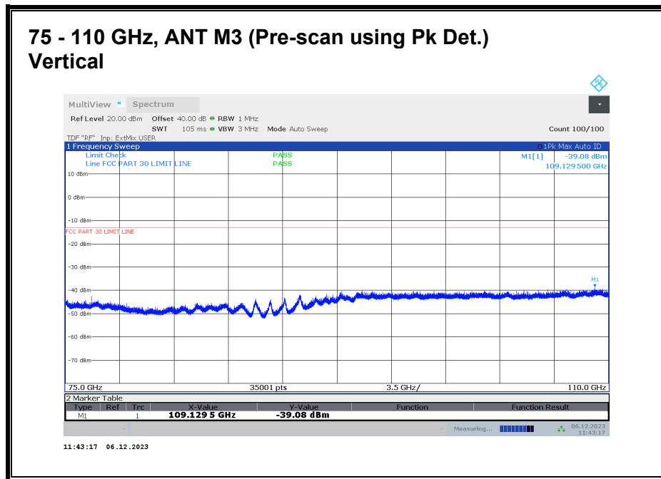
No emission detected using Peak Detection.
