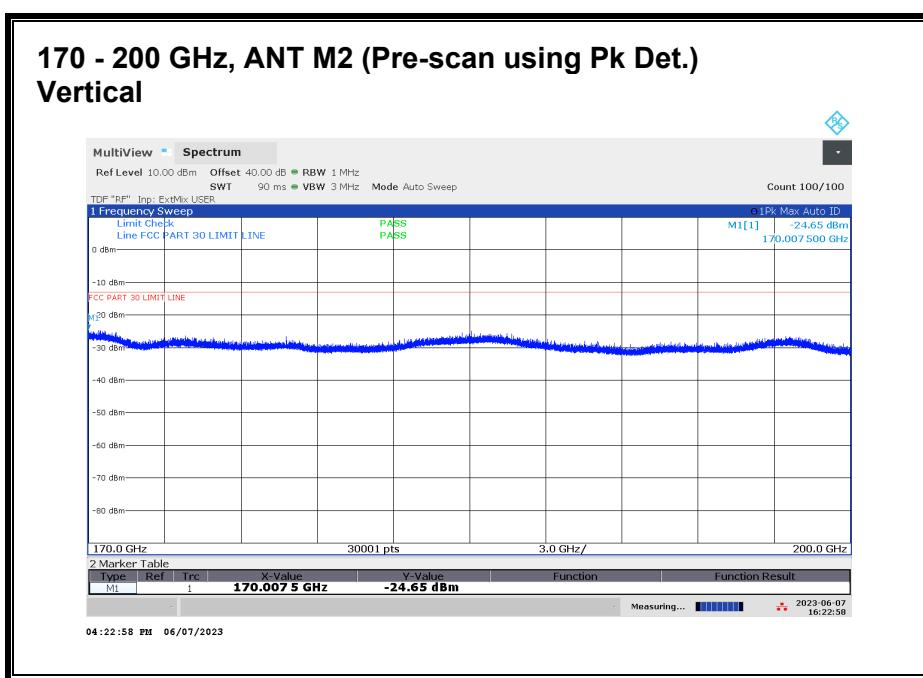
No emission detected using Peak Detection.
