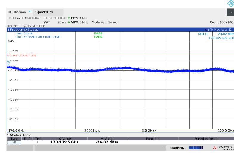
No emission detected using Peak Detection.
