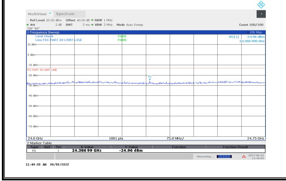
Emissions detected using Peak Detection at pre-scan. Avg EIRP was measured.
