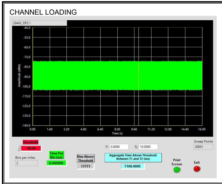
The level of traffic loading on the channel by the EUT is 71.08%
