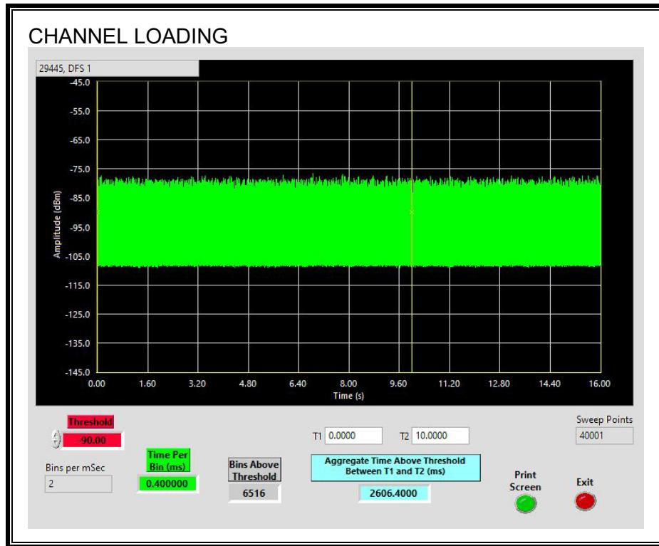
The level of traffic loading on the channel by the EUT is 26.06%
