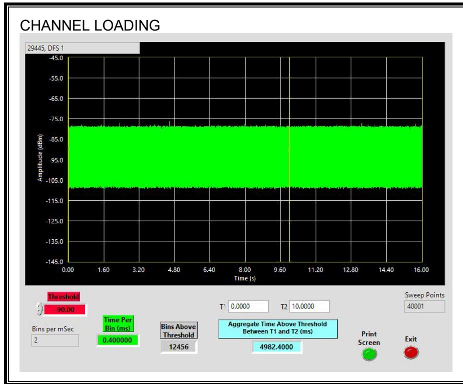
The level of traffic loading on the channel by the EUT is 49.82%
