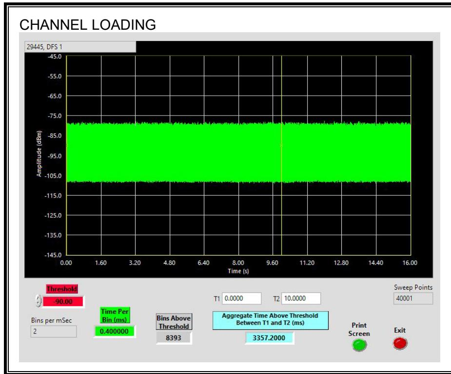
The level of traffic loading on the channel by the EUT is 33.57%
