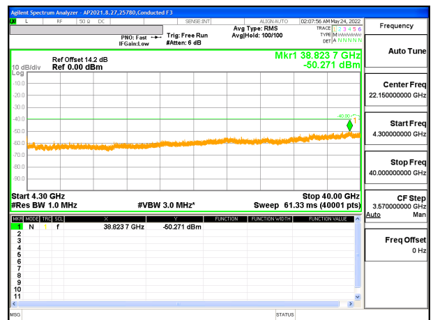
LTE B48 20MHz + 20MHz QPSK Middle Ch RB1-99 + RB1-0 (4.5GHz to 40GHz)
