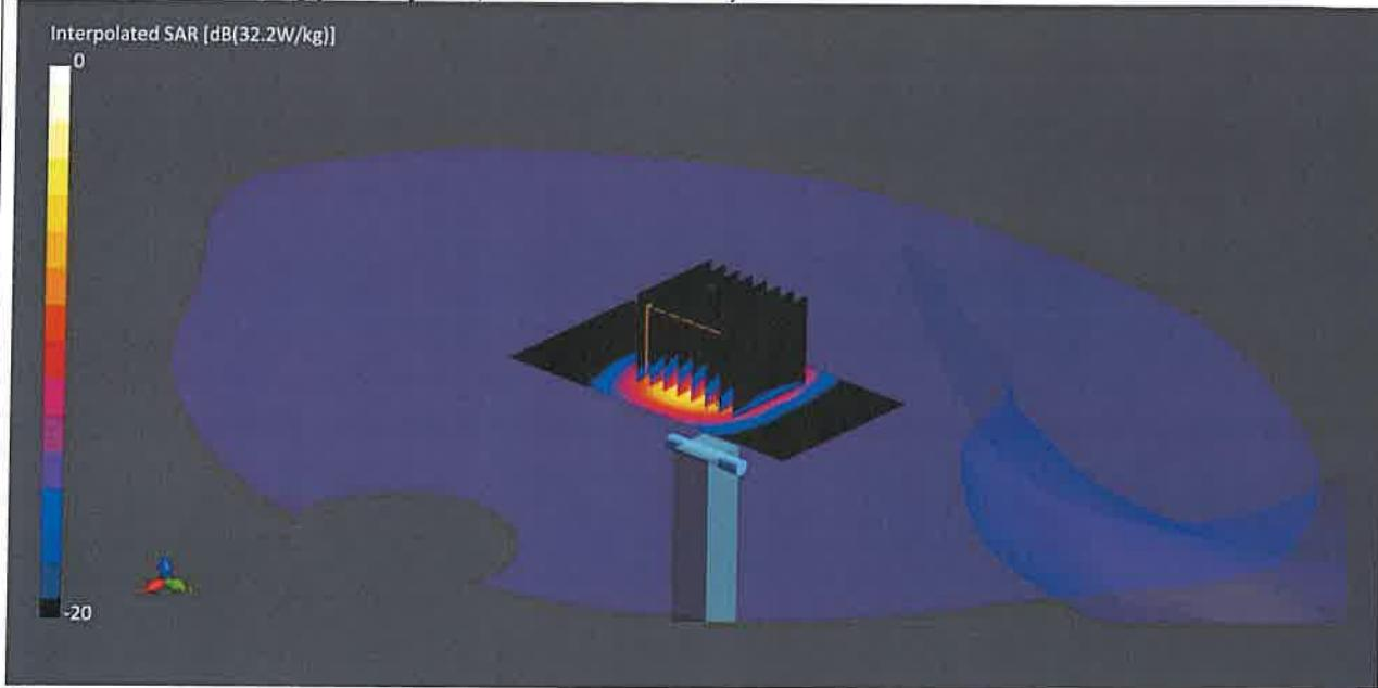
Communication System: CW UID: 0; Frequency: 5750.0 MHz; Duty Cycle: 1;
