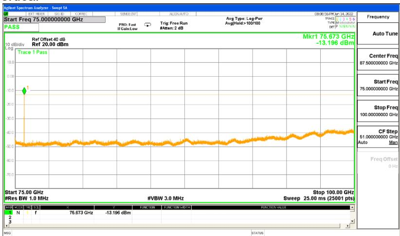
Emissions detected using Peak Detection at pre-scan. Avg EIRP was measured.
