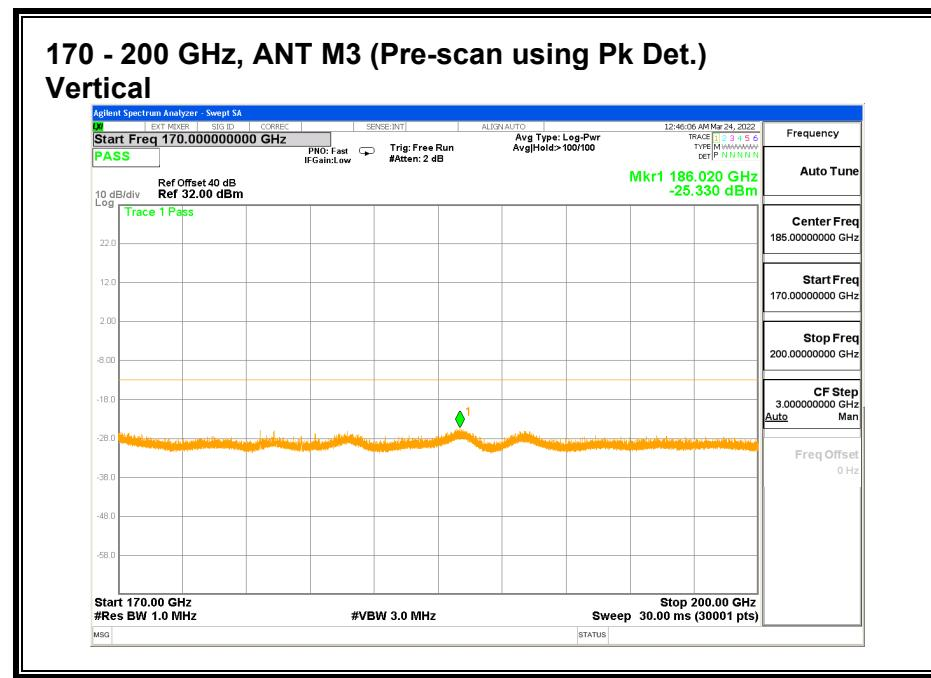
No emission detected using Peak Detection.
