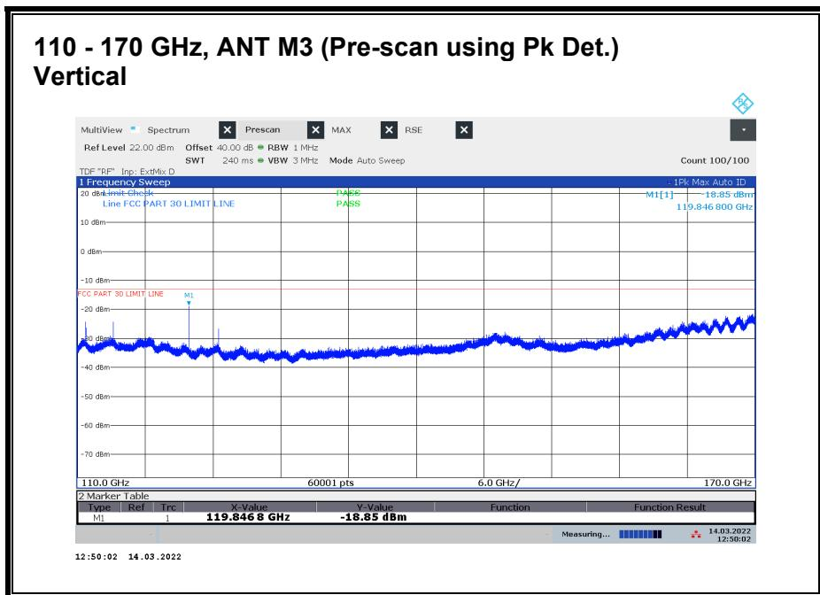
Emissions detected using Peak Detection at pre-scan. Avg EIRP was measured.
