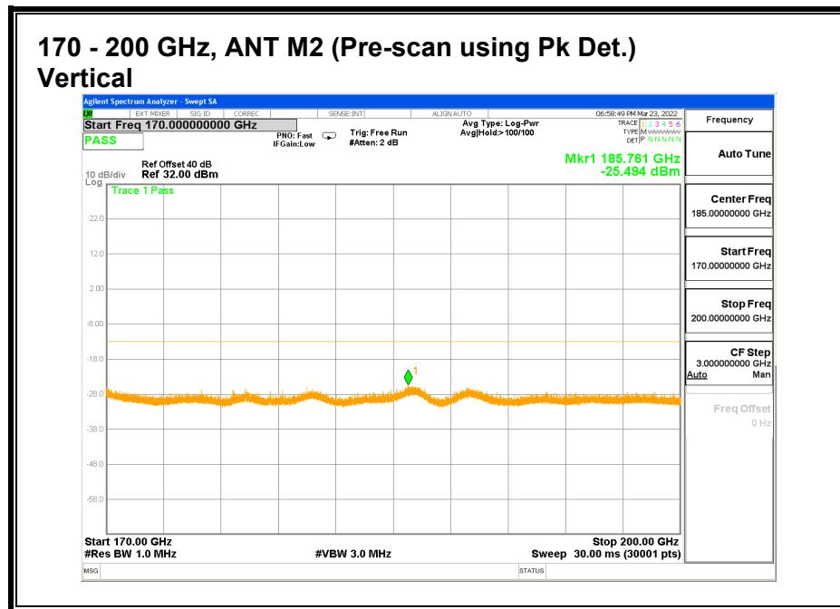
No emission detected using Peak Detection.
