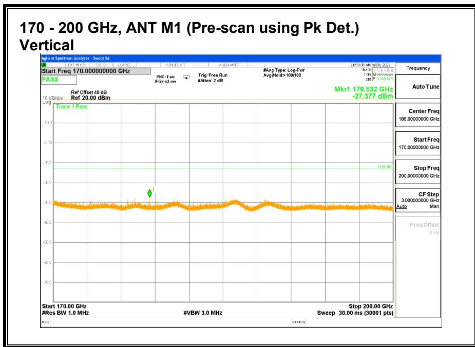
No emission detected using Peak Detection.
