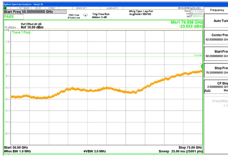
No emission detected using Peak Detection.
