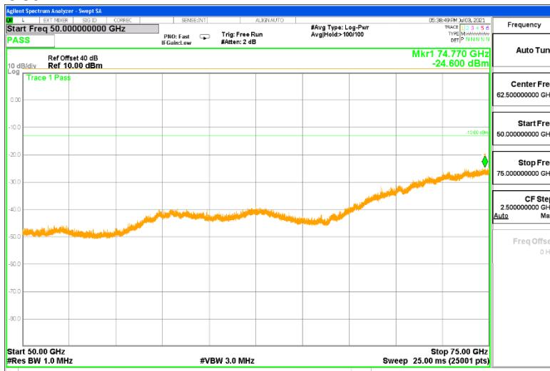
No emission detected using Peak Detection.
