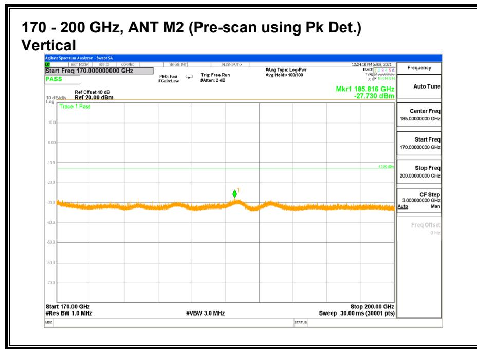
No emission detected using Peak Detection.
