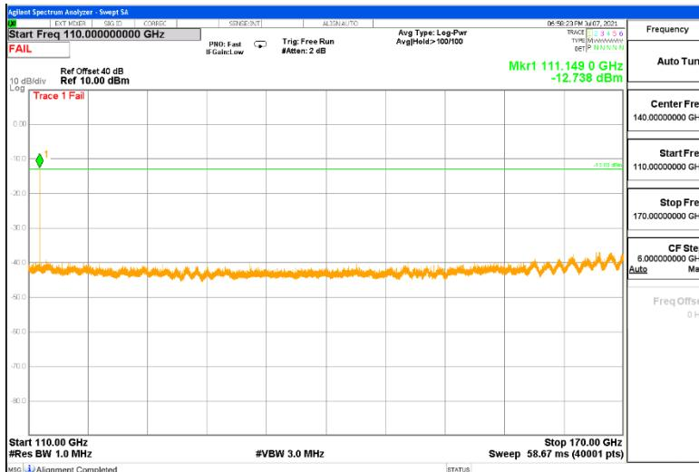
Emissions detected using Peak Detection at pre-scan. Avg EIRP was measured.
