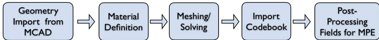
Figure 1. Flowchart of MPE simulation.
