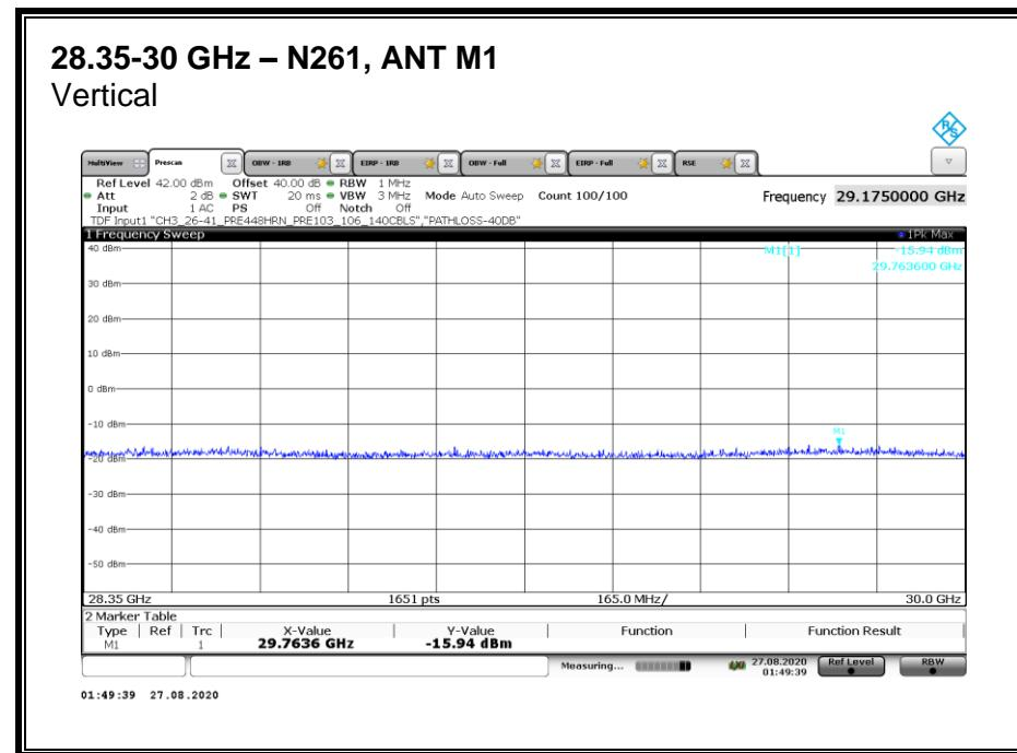
Emission detected using Peak Detection at H-pol. Avg EIRP was measured.
