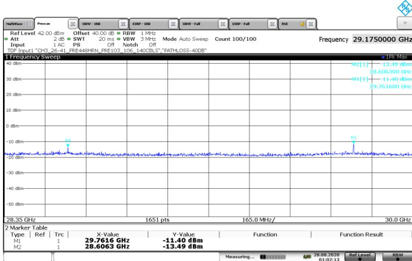
Emissions detected using Peak Detection. Avg EIRP was measured.
