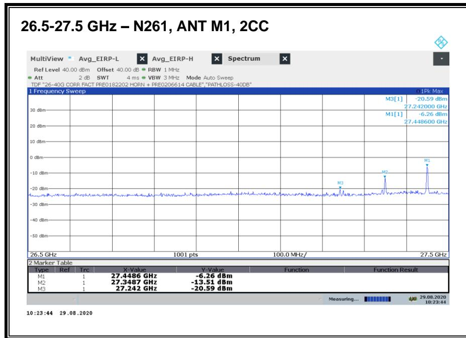
Emissions detected using Peak Detection. Avg EIRP and TRP were measured on highest emission.
