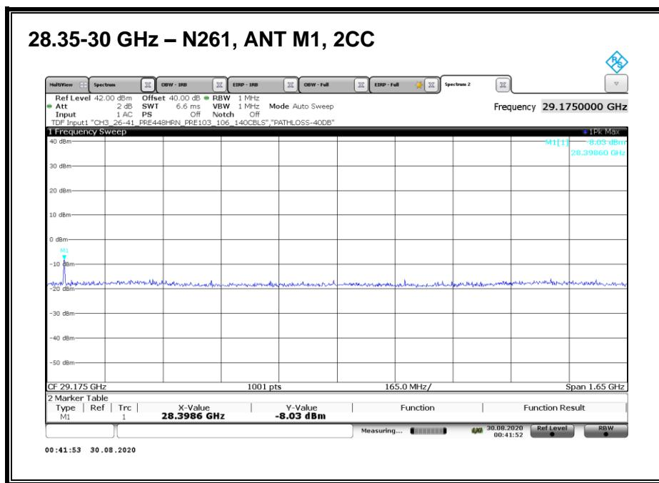
Emissions detected using Peak Detection. Avg EIRP was measured.
