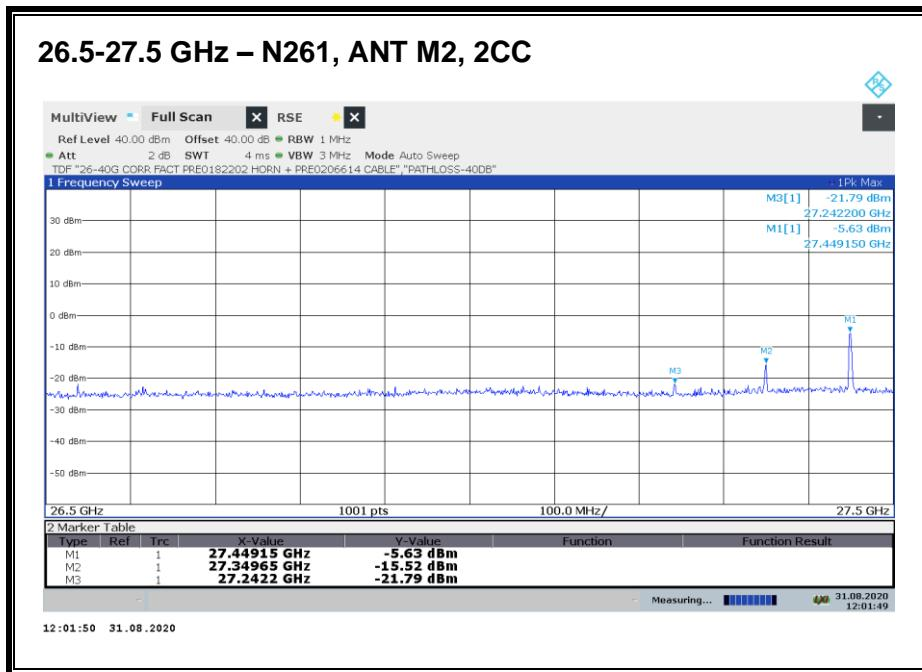
Emission detected using Peak Detection. Avg EIRP and TRP were measured on highest emission.
