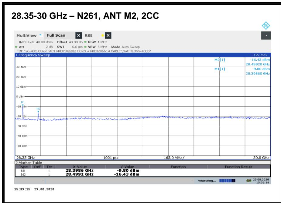
Emission detected using Peak Detection. Avg EIRP was measured on highest emission.
