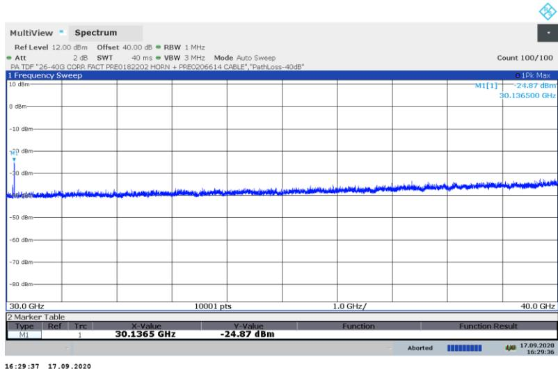
Emissions detected using Peak Detection. Avg EIRP was measured.
