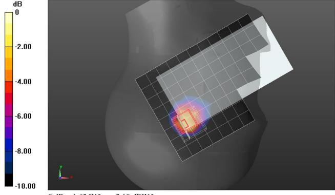
Frequency: 1712.4 MHz; Duty Cycle: 1:1; Room Ambient Temperature: 24.0°C; Liquid Temperature: 23.0°C Medium parameters used (interpolated): f = 1712.4 MHz;  $\sigma = 1.403$  S/m;  $\epsilon_r = 38.248$ ;  $\rho = 1000$  kg/m³ DASY5 Configuration:
