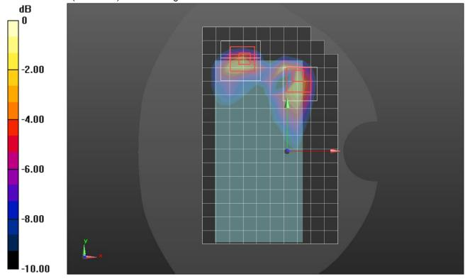
Frequency: 2549.5 MHz; Duty Cycle: 1:1.59956; Room Ambient Temperature: 24.0°C; Liquid Temperature: 23.0°C Medium parameters used: f = 2550 MHz;  $\sigma$  = 1.983 S/m;  $\epsilon_r$  = 38.25;  $\rho$  = 1000 kg/m³ DASY5 Configuration:
