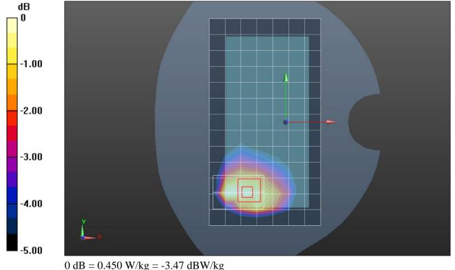
Frequency: 836.6 MHz; Duty Cycle: 1:4.00037; Room Ambient Temperature: 24.0°C; Liquid Temperature: 23.0°C Medium parameters used (interpolated): f = 836.6 MHz;  $\sigma = 0.929$  S/m;  $\epsilon_r = 42.949$ ;  $\rho = 1000$  kg/m³ DASY5 Configuration:
