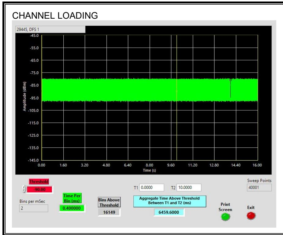
The level of traffic loading on the channel by the EUT is 64.59%
