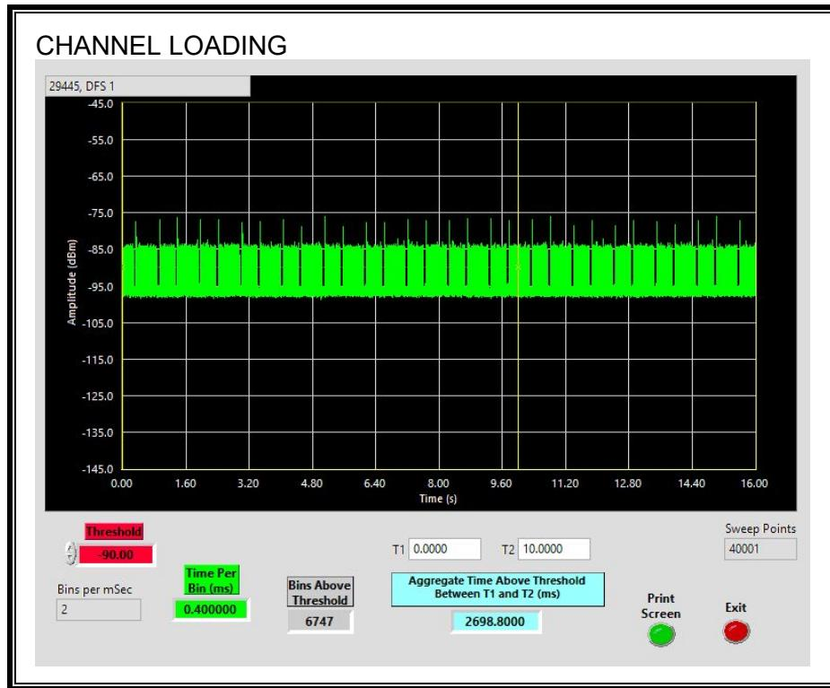
The level of traffic loading on the channel by the Peer Slave is 26.98%
