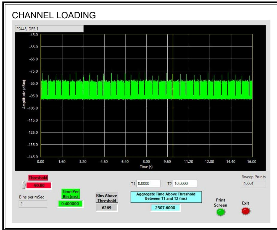
The level of traffic loading on the channel by the Peer Slave is 25.07%
