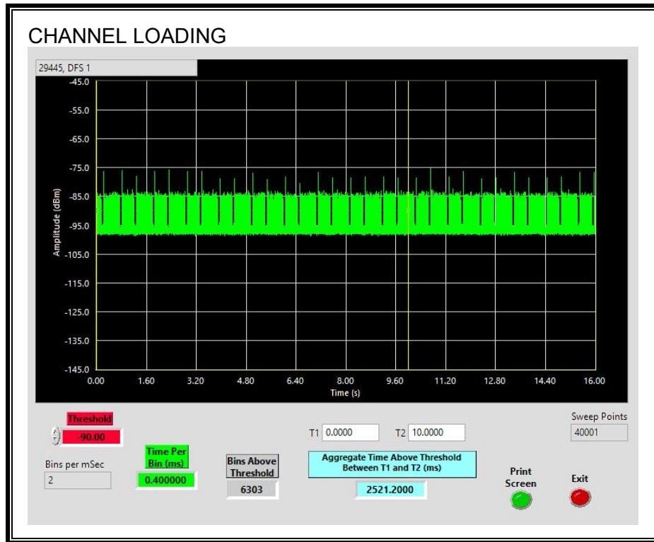
The level of traffic loading on the channel by the Peer Slave is 25.21%
