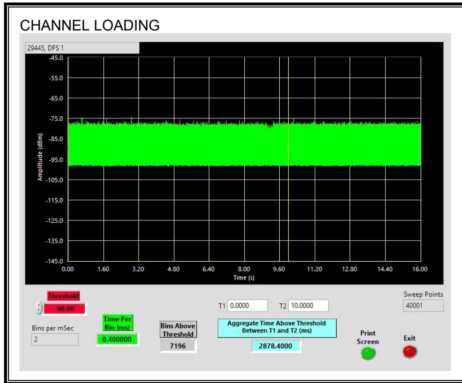
The level of traffic loading on the channel by the EUT is 28.78%
