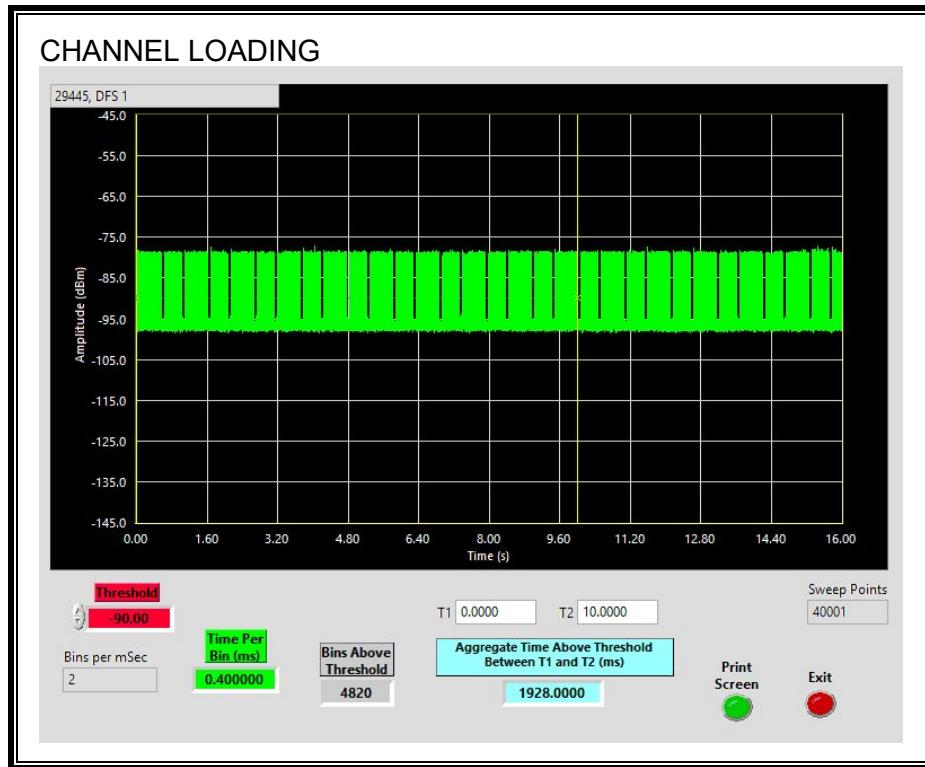
The level of traffic loading on the channel by the EUT is 19.28%
