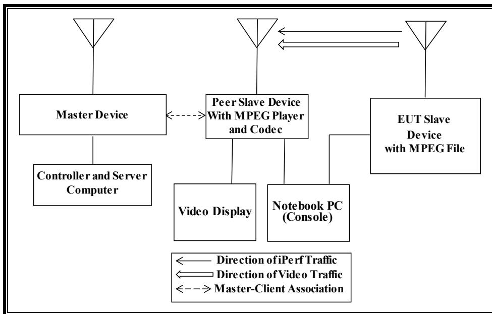
**RADIATED METHOD EUT TEST SETUP WHEN MONITORING THE PEER SLAVE DEVICE)**
