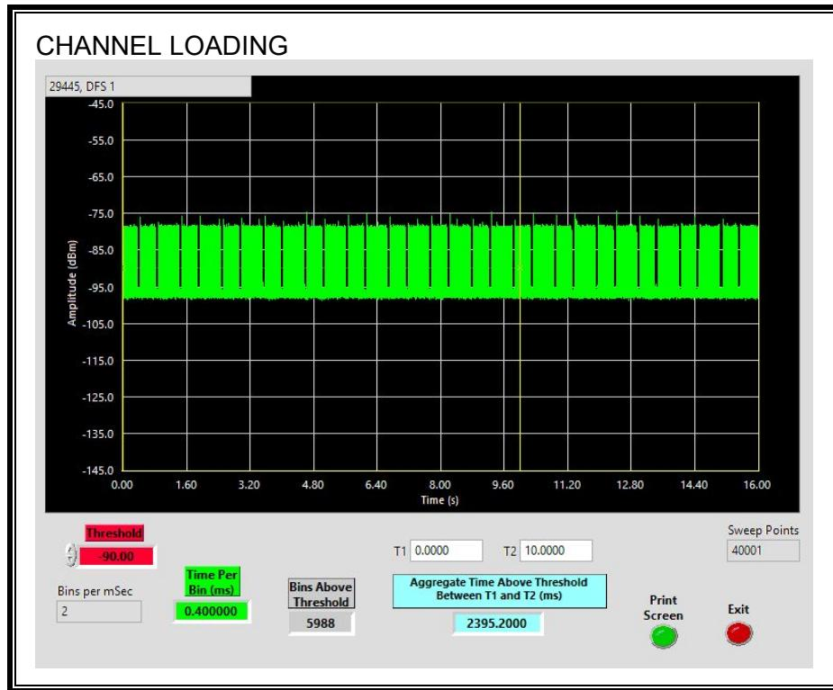
The level of traffic loading on the channel by the EUT is 23.95%
