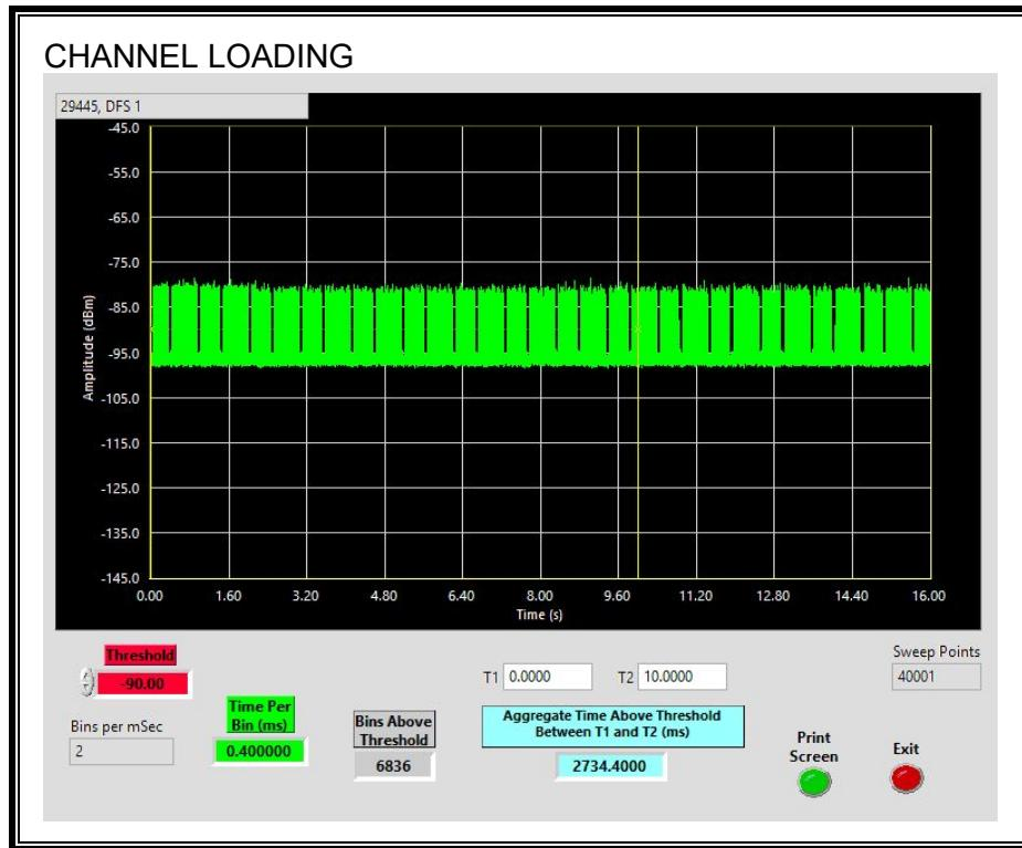
The level of traffic loading on the channel by the EUT is 27.34%
