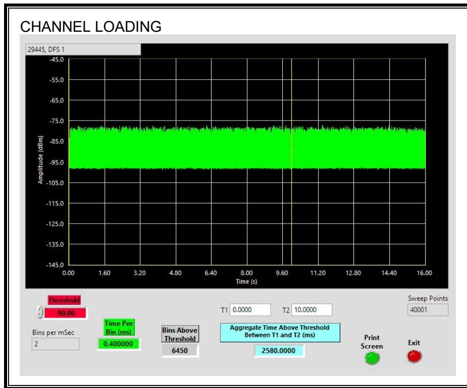
The level of traffic loading on the channel by the EUT is 25.8%
