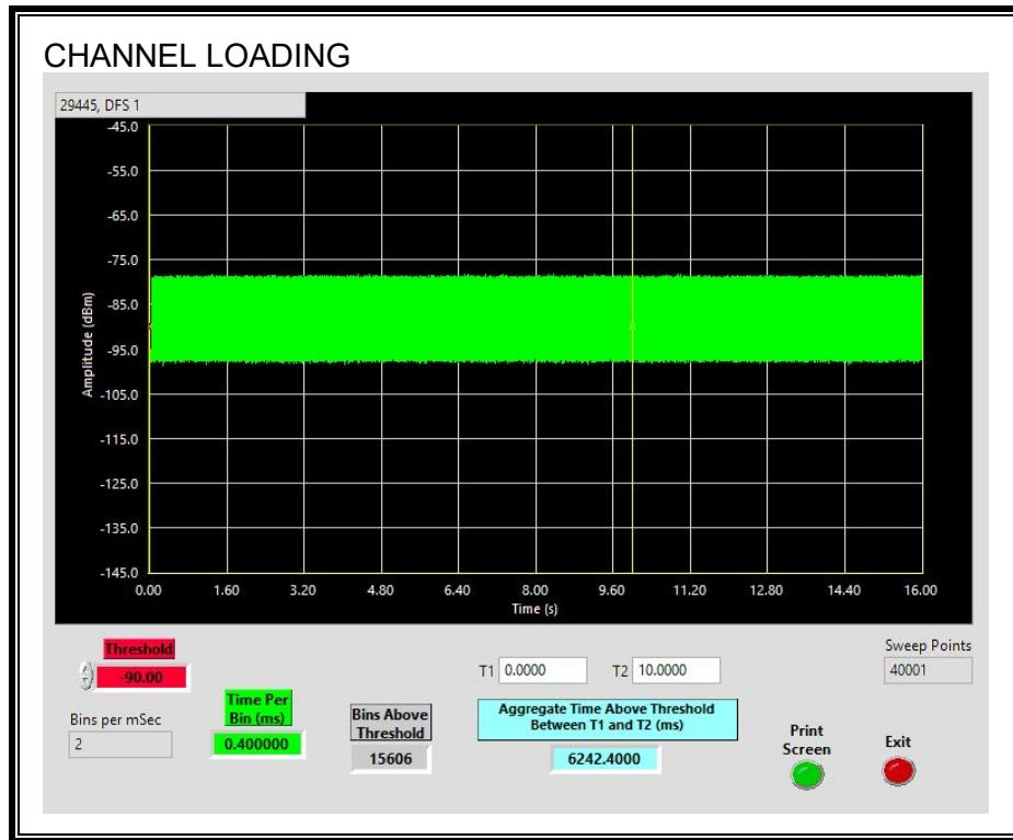
The level of traffic loading on the channel by the EUT is 62.42%
