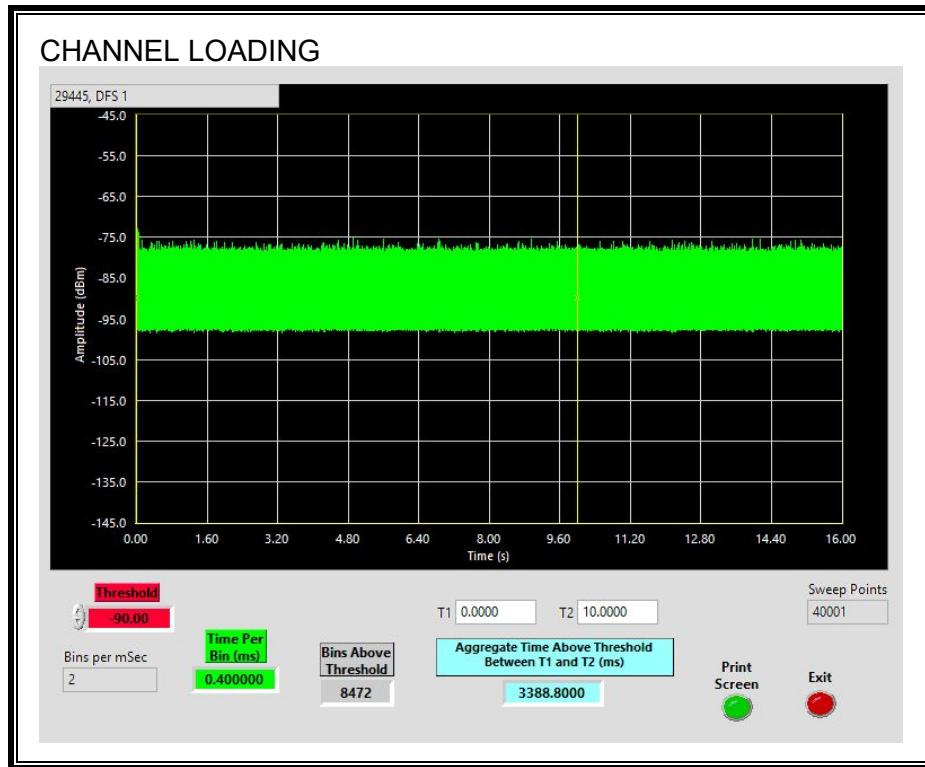
The level of traffic loading on the channel by the EUT is 33.88%
