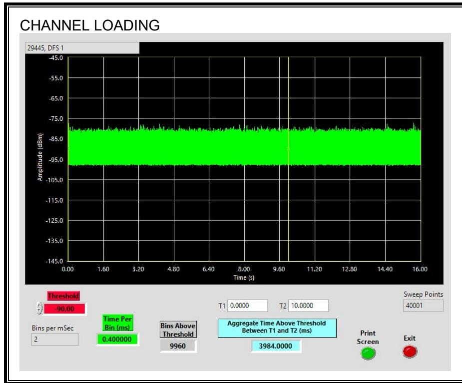
The level of traffic loading on the channel by the EUT is 39.84%
