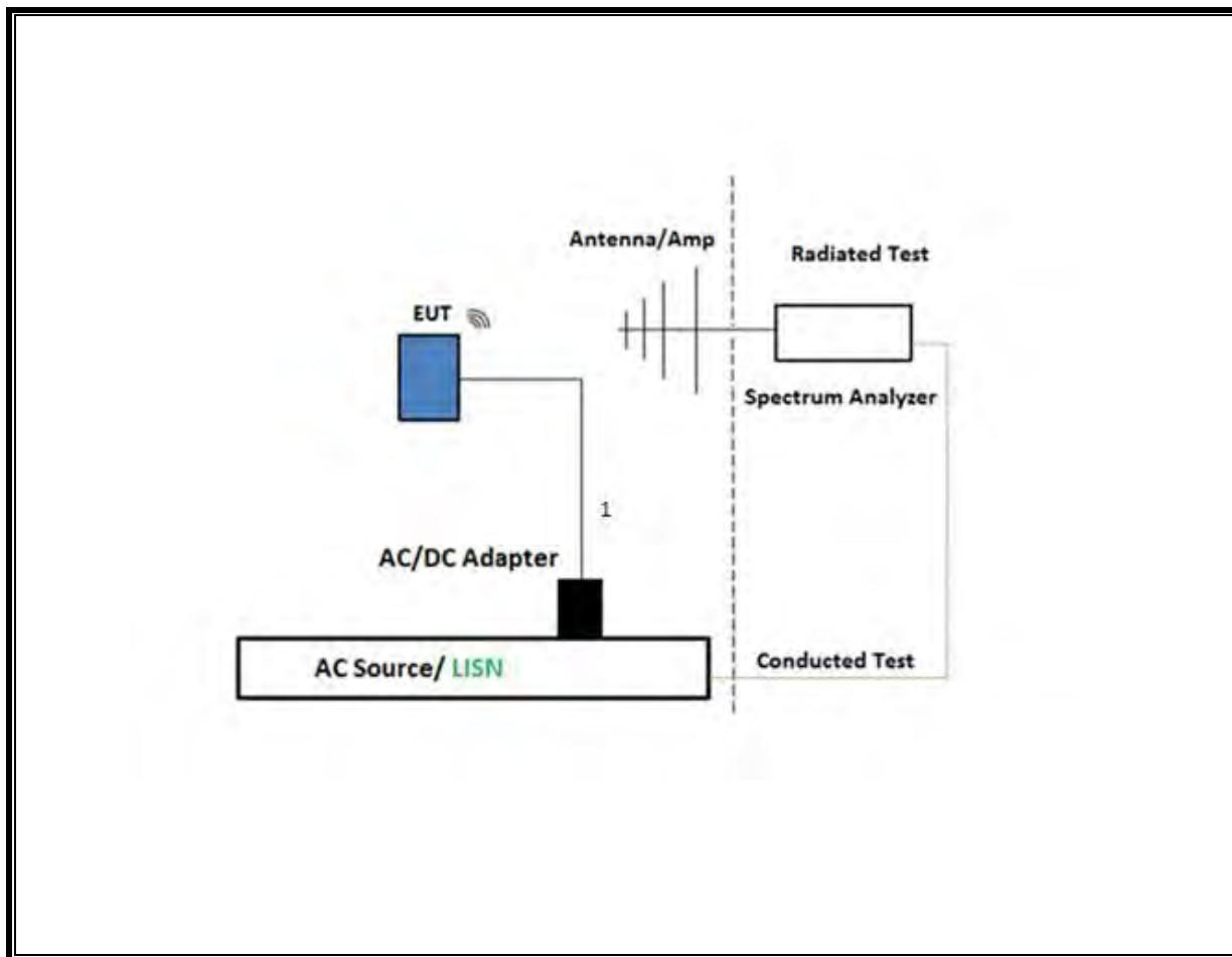
**TEST SETUP- AC LINE CONDUCTED: LAPTOP CONFIGURATION**
