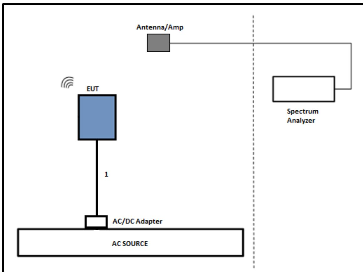
**SETUP DIAGRAM FOR LINE CONDUCTED TESTS**
