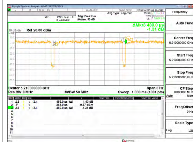
DUTY CYCLE 802.11ac VHT80 1Tx MODE
