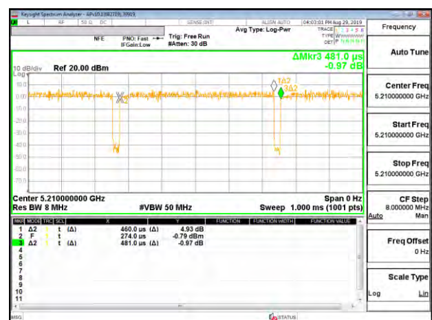
DUTY CYCLE 802.11ac VHT80 2TX CDD MODE
