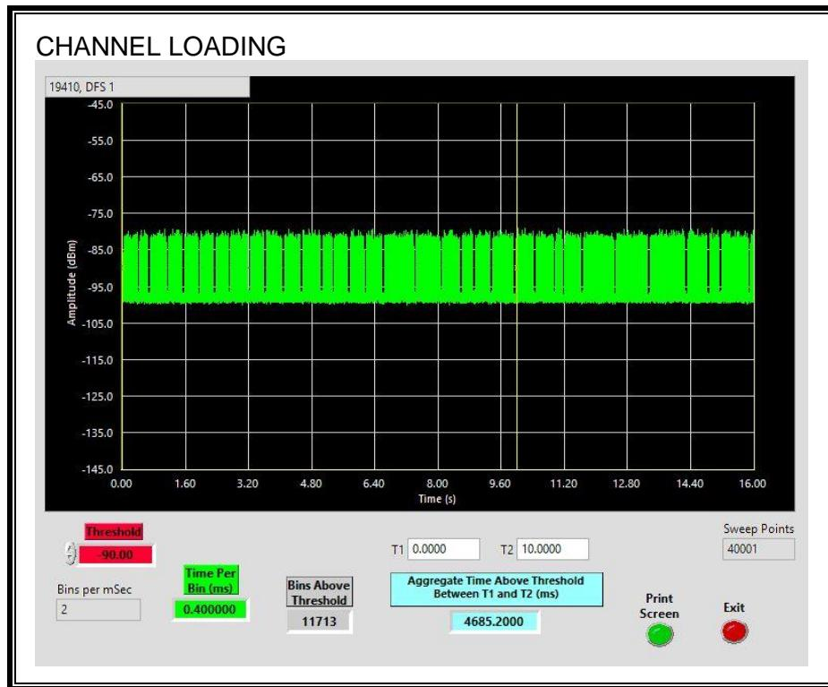
The level of traffic loading on the channel by the EUT is 46.85%
