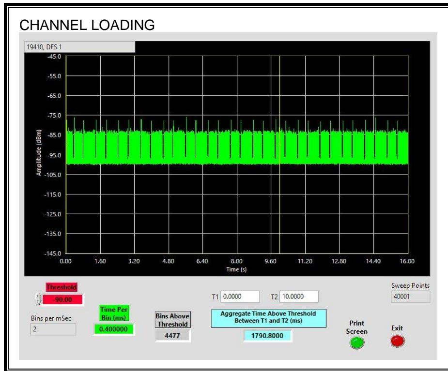
The level of traffic loading on the channel by the Peer Slave is 17.90%
