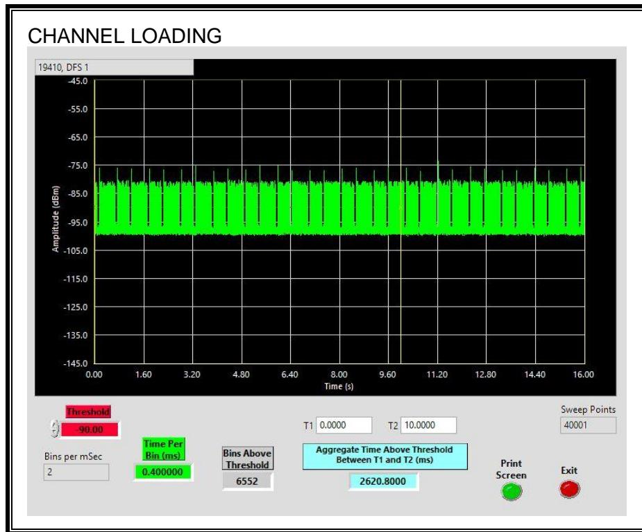
The level of traffic loading on the channel by the Peer Slave is 26.20%
