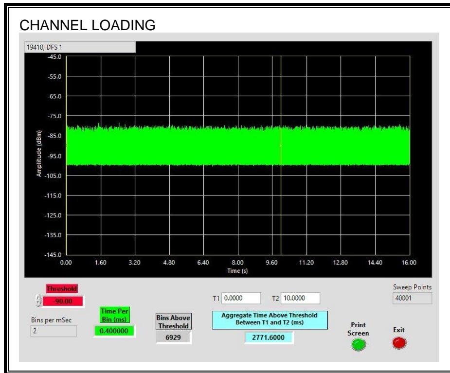
The level of traffic loading on the channel by the EUT is 27.71%
