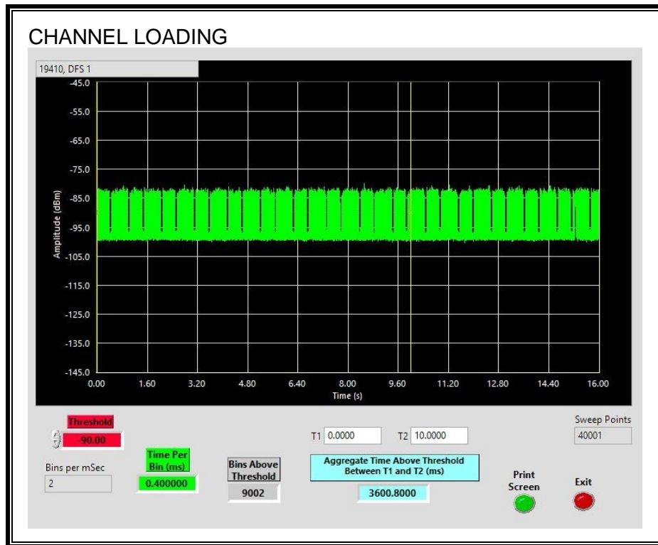
The level of traffic loading on the channel by the EUT is 36.00%
