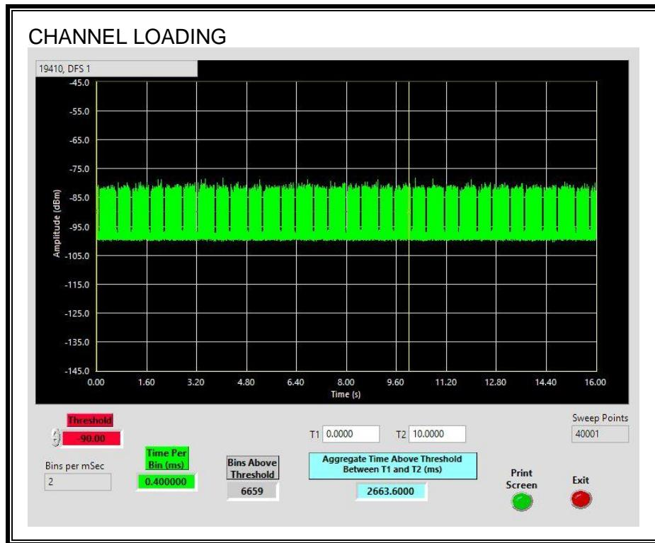
The level of traffic loading on the channel by the EUT is 26.63%
