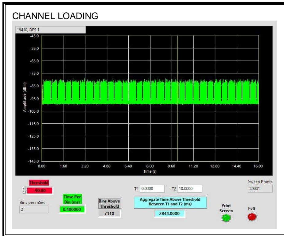
The level of traffic loading on the channel by the EUT is 28.44%
