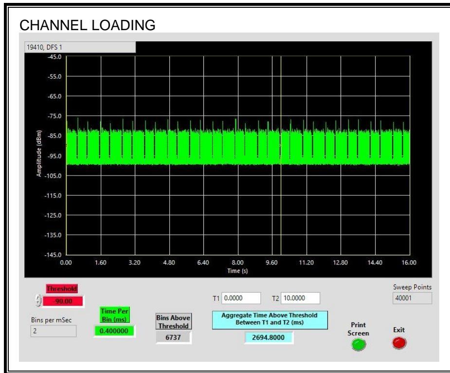
The level of traffic loading on the channel by the Peer Slave is 26.94%
