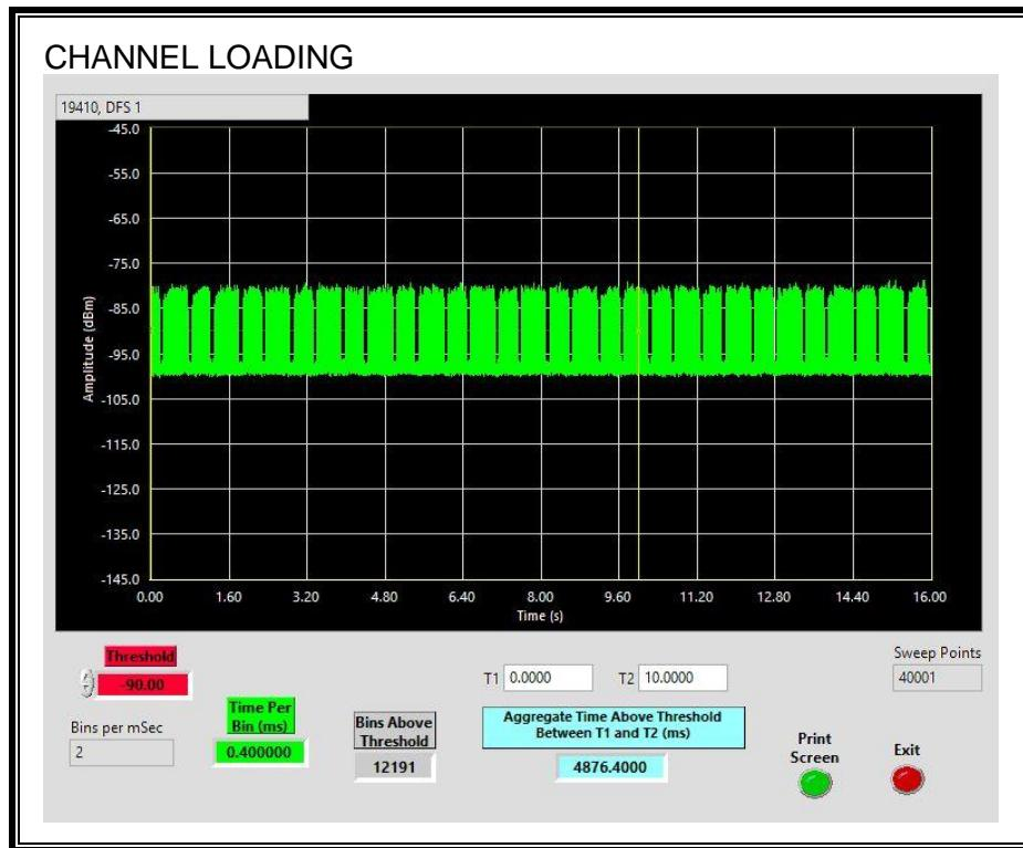
The level of traffic loading on the channel by the EUT is 48.76%
