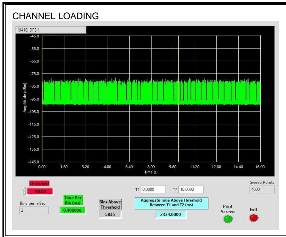
The level of traffic loading on the channel by the EUT is 23.34%
