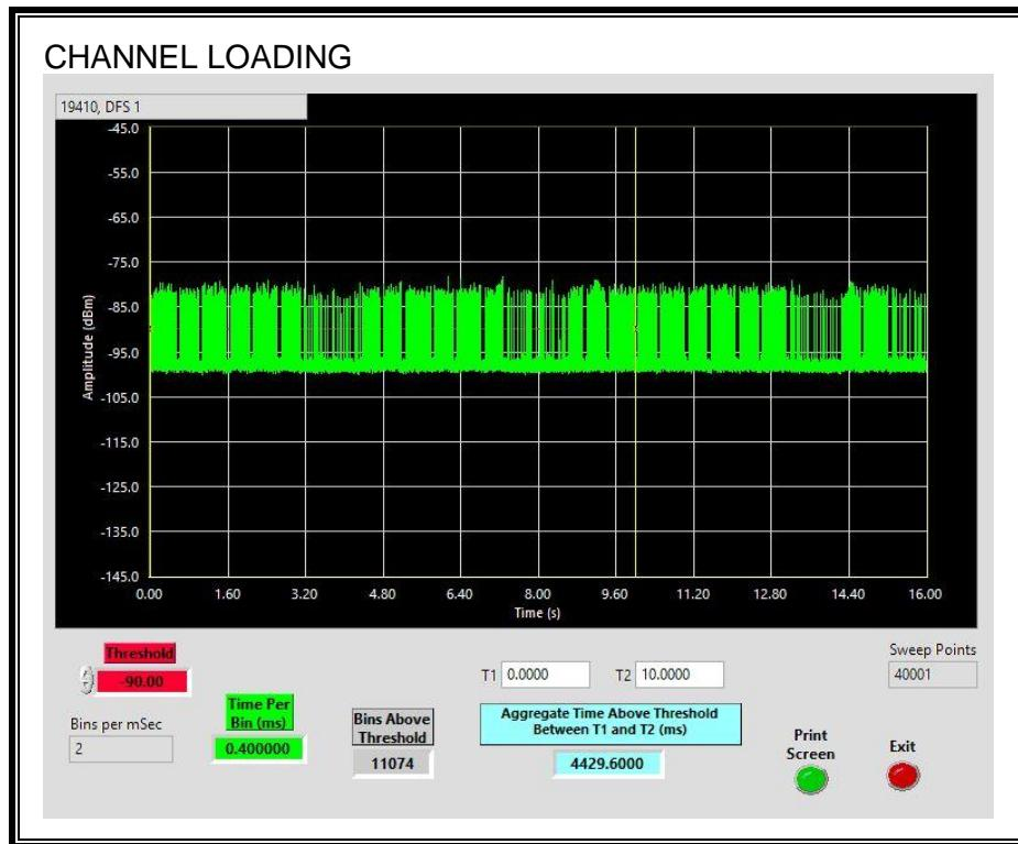
The level of traffic loading on the channel by the EUT is 44.29%
