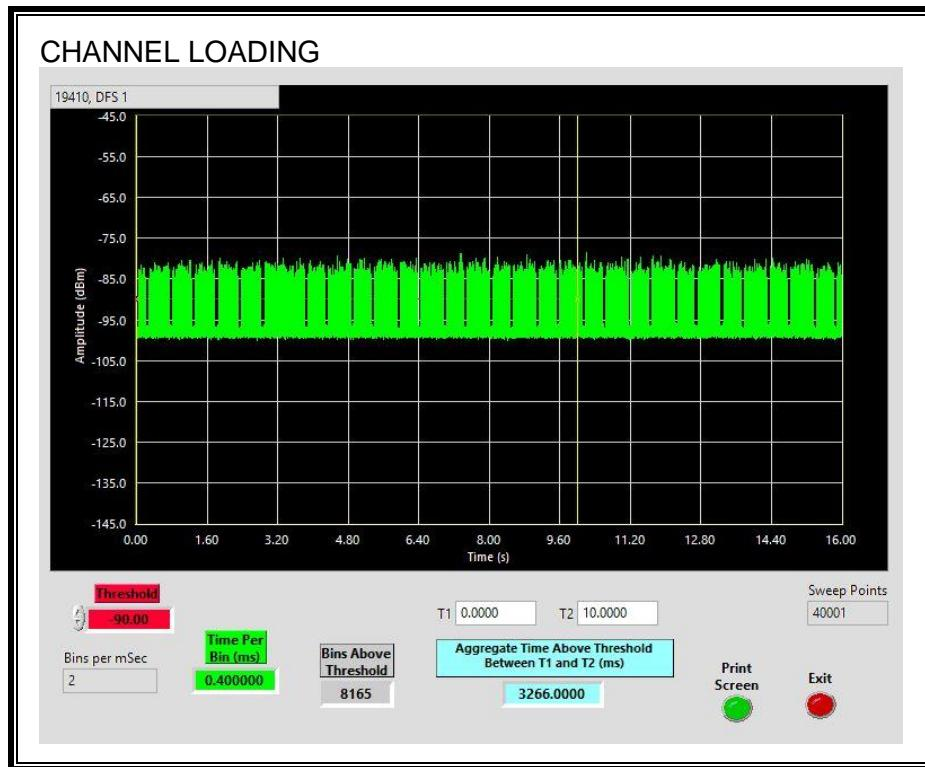
The level of traffic loading on the channel by the EUT is 32.66%
